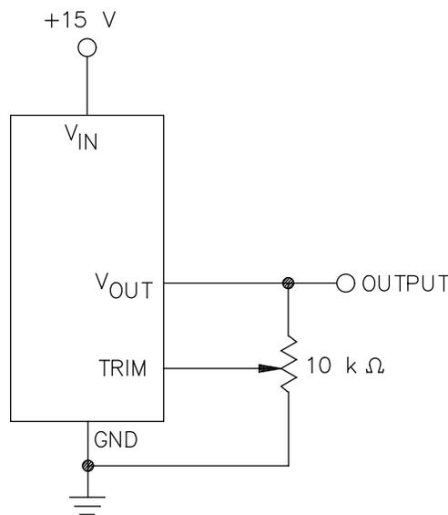
FIGURE 2.  $V_{OUT}$  trim circuit.
