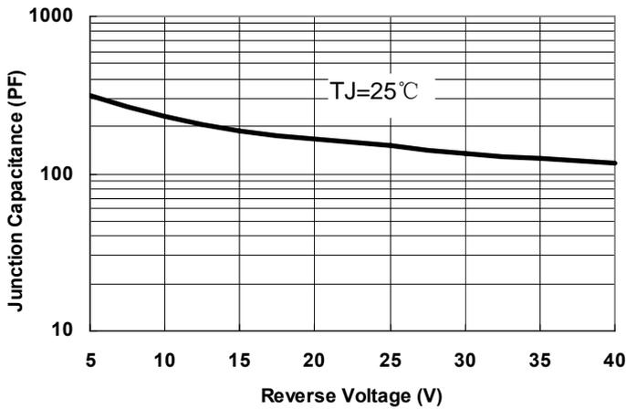
Fig.1-Typical Junction Capacitance
