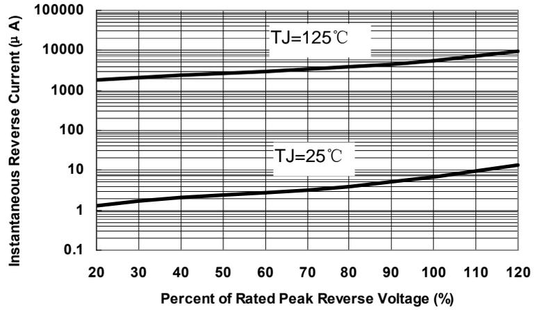
Fig.2-Typical Reverse Characteristics
