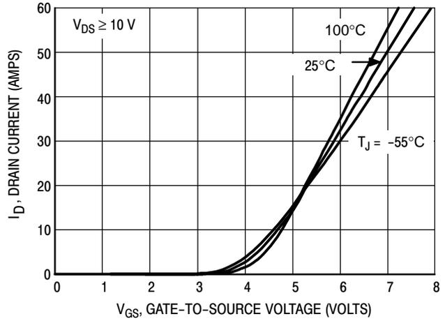
Figure 2. Transfer Characteristics
