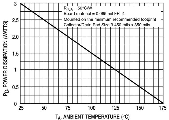
Figure 15. D<sup>2</sup>PAK Power Derating Curve
