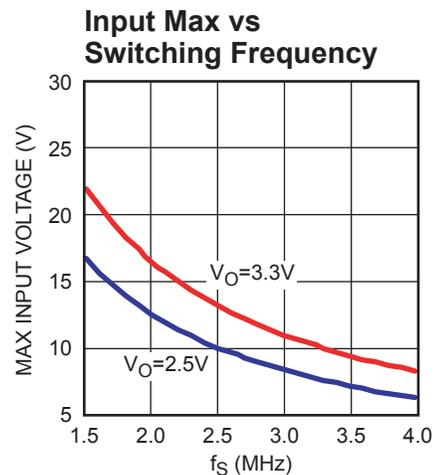
**Figure 2—Recommended Input vs. f<sub>s</sub>**
