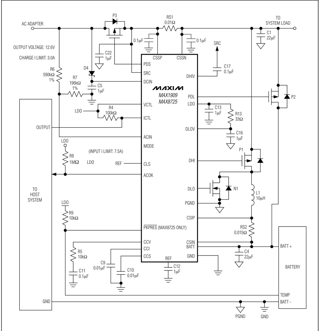
Figure 1. Typical Operating Circuit Demonstrating Hardwired Control
