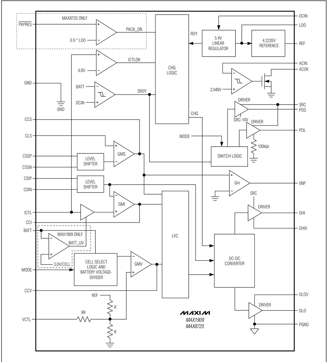
Figure 3. Functional Diagram
