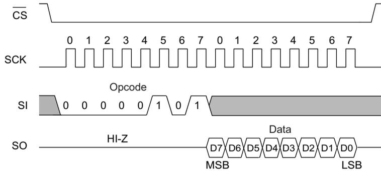
Figure 9. WRSR Bus Configuration (WREN not shown)
