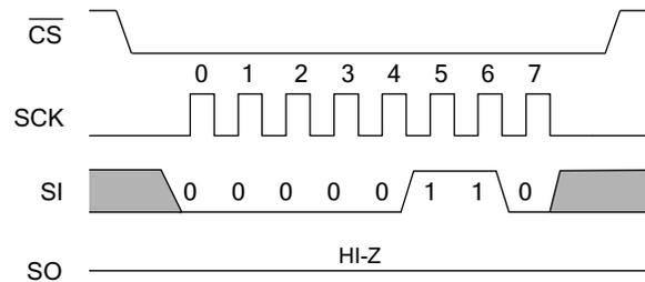
**WRDI - Reset Write Enable Latch**
