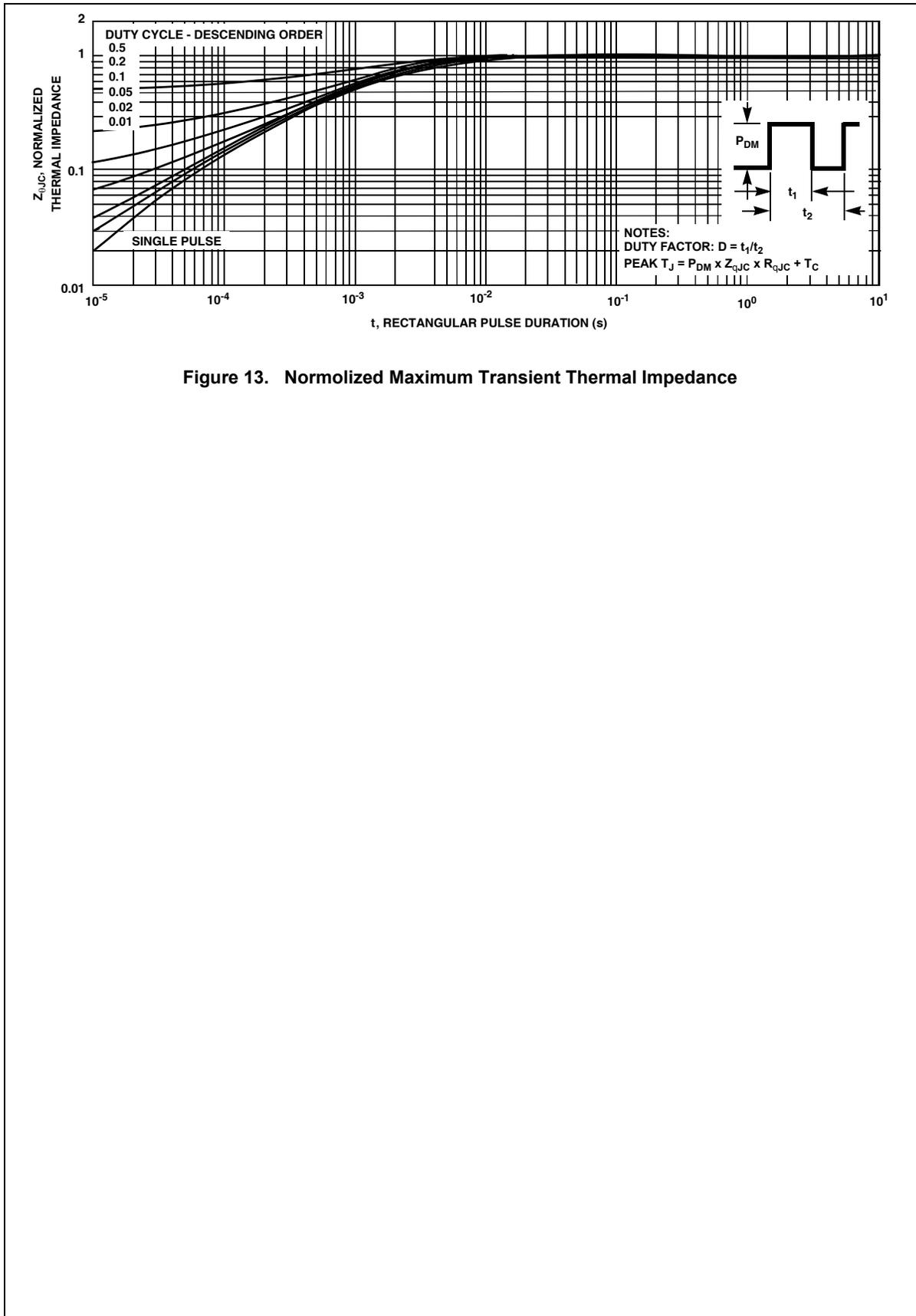
Figure 13. Normalized Maximum Transient Thermal Impedance
