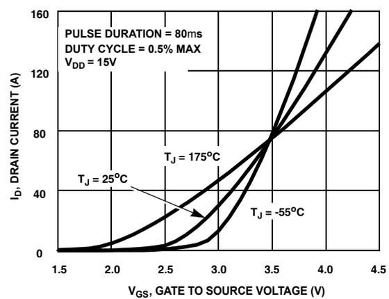
Figure 5. Transfer Characteristics
