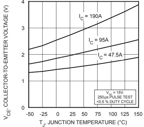
**FIGURE 5, On State Voltage vs Junction Temperature**
