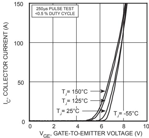
**FIGURE 6, Transfer Characteristics**
