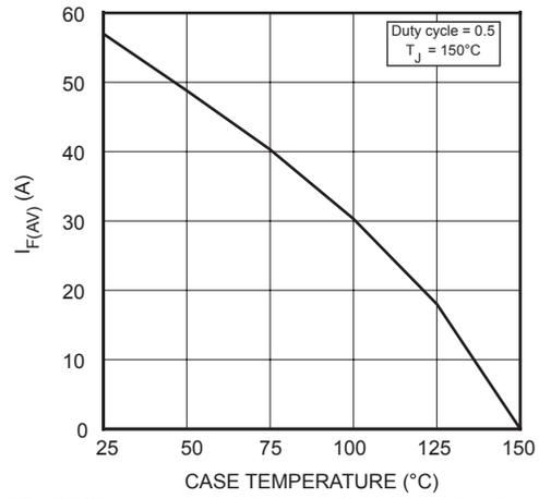
**FIGURE 24, Max Average Forward Current vs. Case Temperature**
