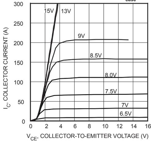
**FIGURE 4, Output Characteristics ( $T_J = 25^{\circ}C$ )**
