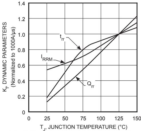
**FIGURE 23, Dynamic Parameters vs. Junction Temperature**
