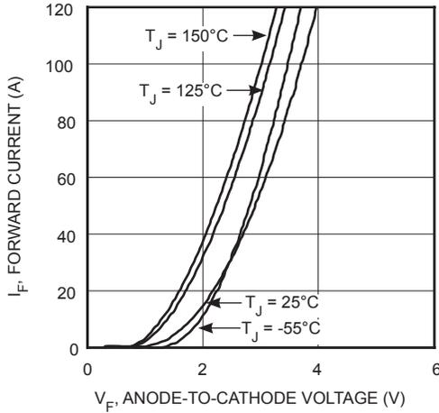
**FIGURE 19, F Forward Current vs. Forward Voltage**
