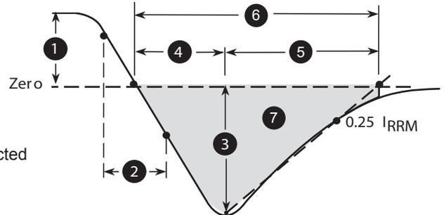
FIGURE 26. Diode Reverse Recovery Waveform Definition
