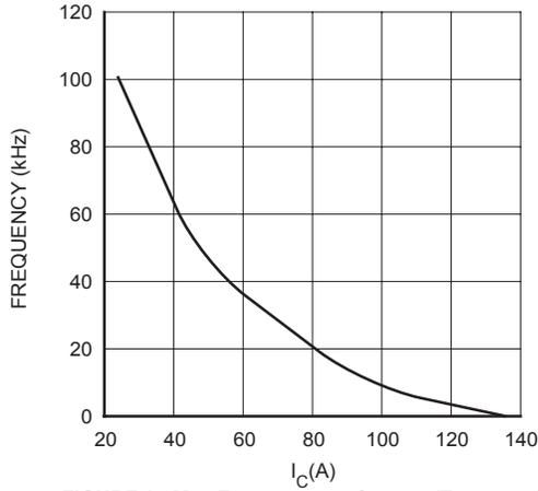
**FIGURE 2, Max Frequency vs Current ( $T_{case} = 75^{\circ}C$ )**
