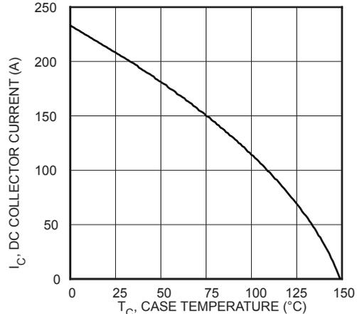
**FIGURE 9, DC Collector Current vs Case Temperature**
