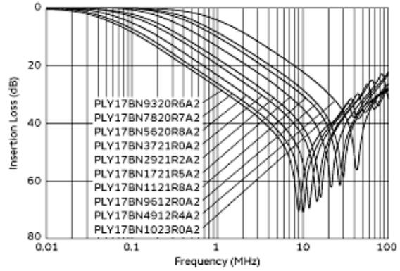
Differential Mode Insertion Loss-Frequency Characteristics
