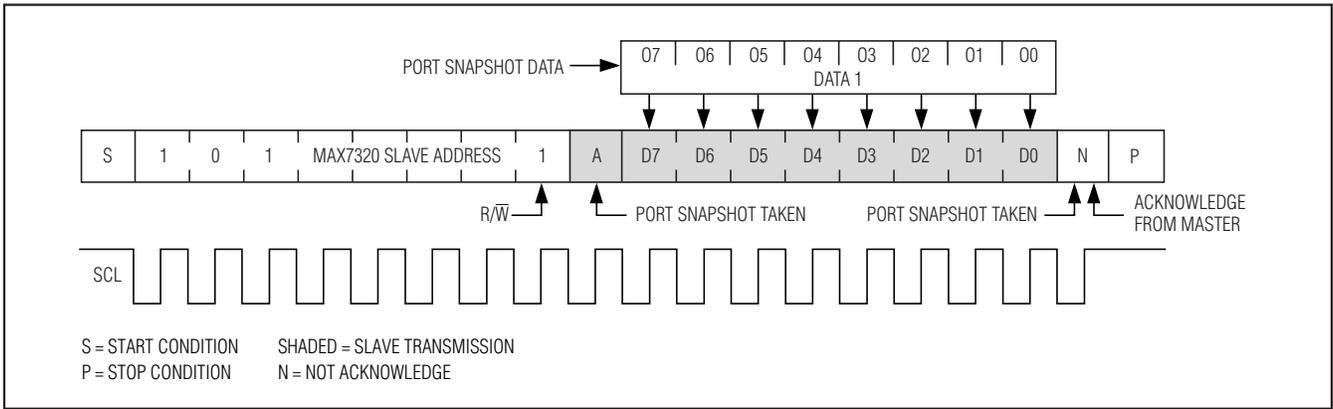
Figure 6. Reading the MAX7320
