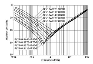
Common Mode Insertion Loss (Typ.)
