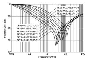
Differential Mode Insertion Loss (Typ.)
