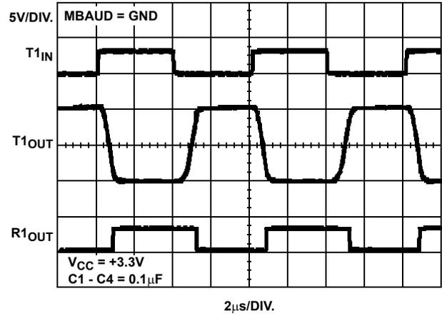
FIGURE 6. LOOPBACK TEST AT 250kbps ( $C_L = 1000\text{pF}$ )
