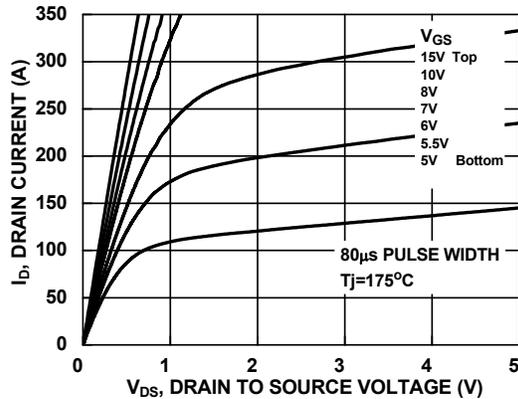
Figure 10. Saturation Characteristics
