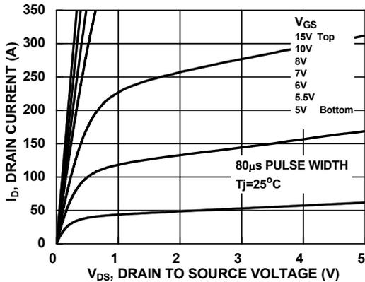
Figure 9. Saturation Characteristics
