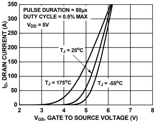
Figure 7. Transfer Characteristics
