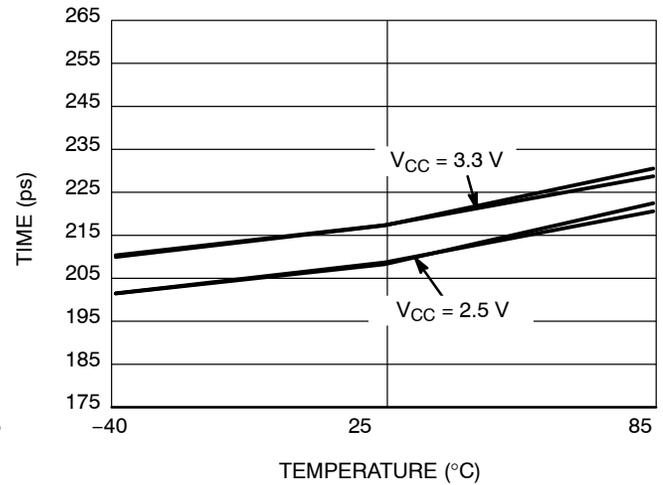
**Figure 6. Propagation Delay vs. Temperature and Power Supply**
