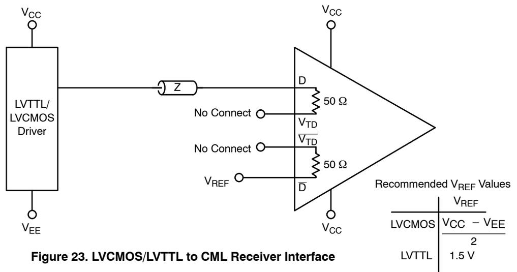
Figure 23. LVCMOS/LVTTL to CML Receiver Interface
