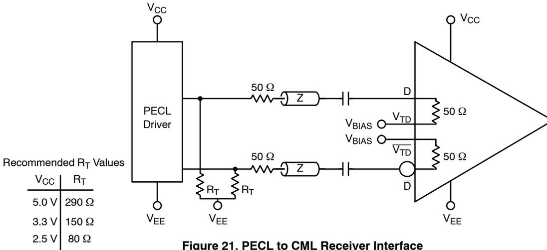
Figure 21. PECL to CML Receiver Interface
