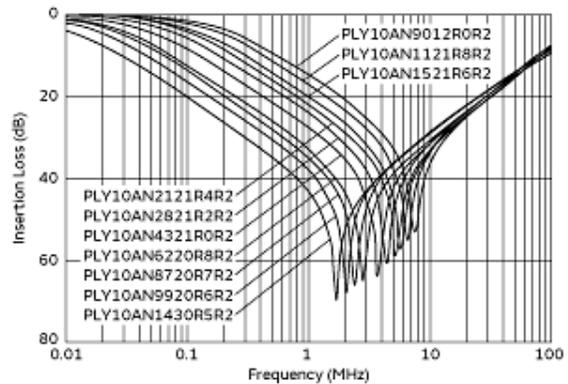
Differential Mode Insertion Loss-Frequency Characteristics
