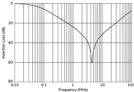
Differential Mode Insertion Loss (Typ.)
