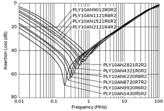
Common Mode Insertion Loss-Frequency Characteristics
