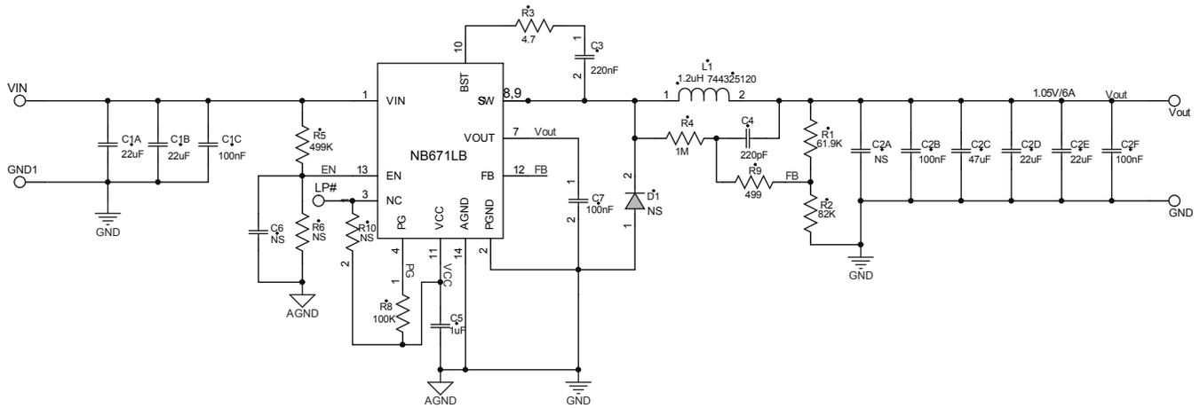
**Figure 14 — Typical Application Circuit For NB671LB**
