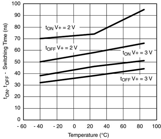
Switching Time vs. Temperature and Supply Voltage
