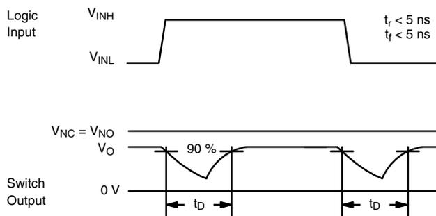
Figure 2. Break-Before-Make Interval
