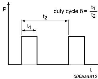
Fig. 14. Duty cycle definition
