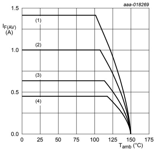
FR4 PCB, mounting pad for anode and cathode 1  $\text{cm}^2$  each
