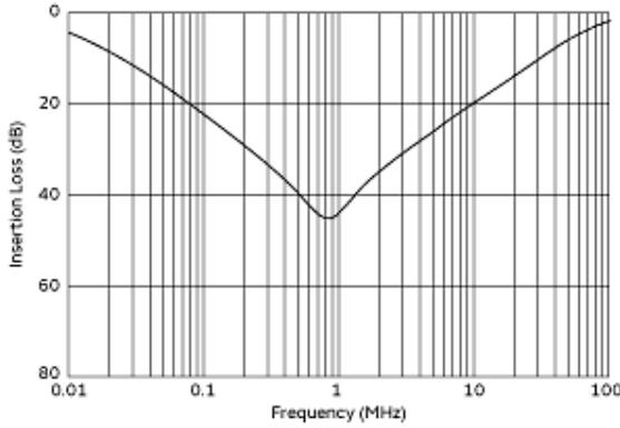
Common Mode Insertion Loss (Typ.)
