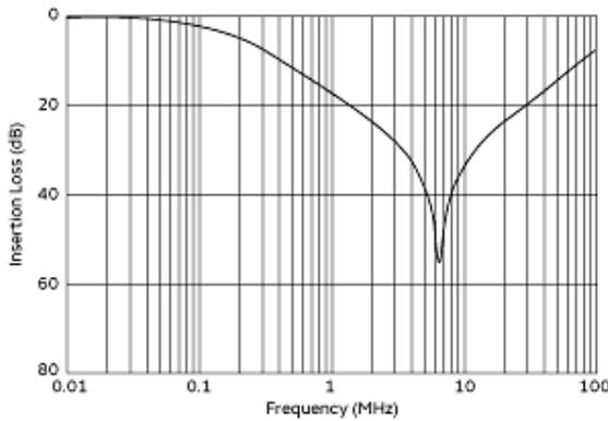
Differential Mode Insertion Loss (Typ.)
