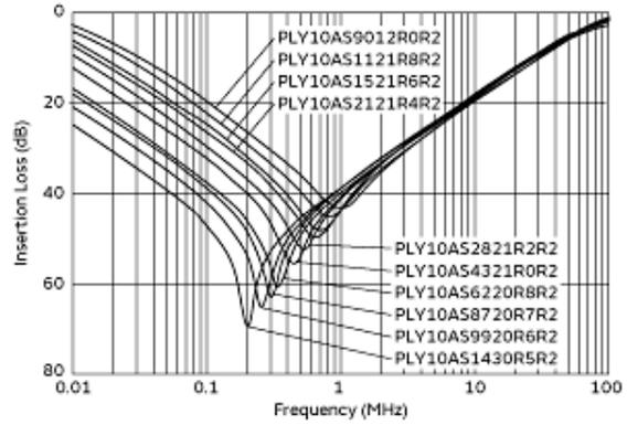
Common Mode Insertion Loss-Frequency Characteristics
