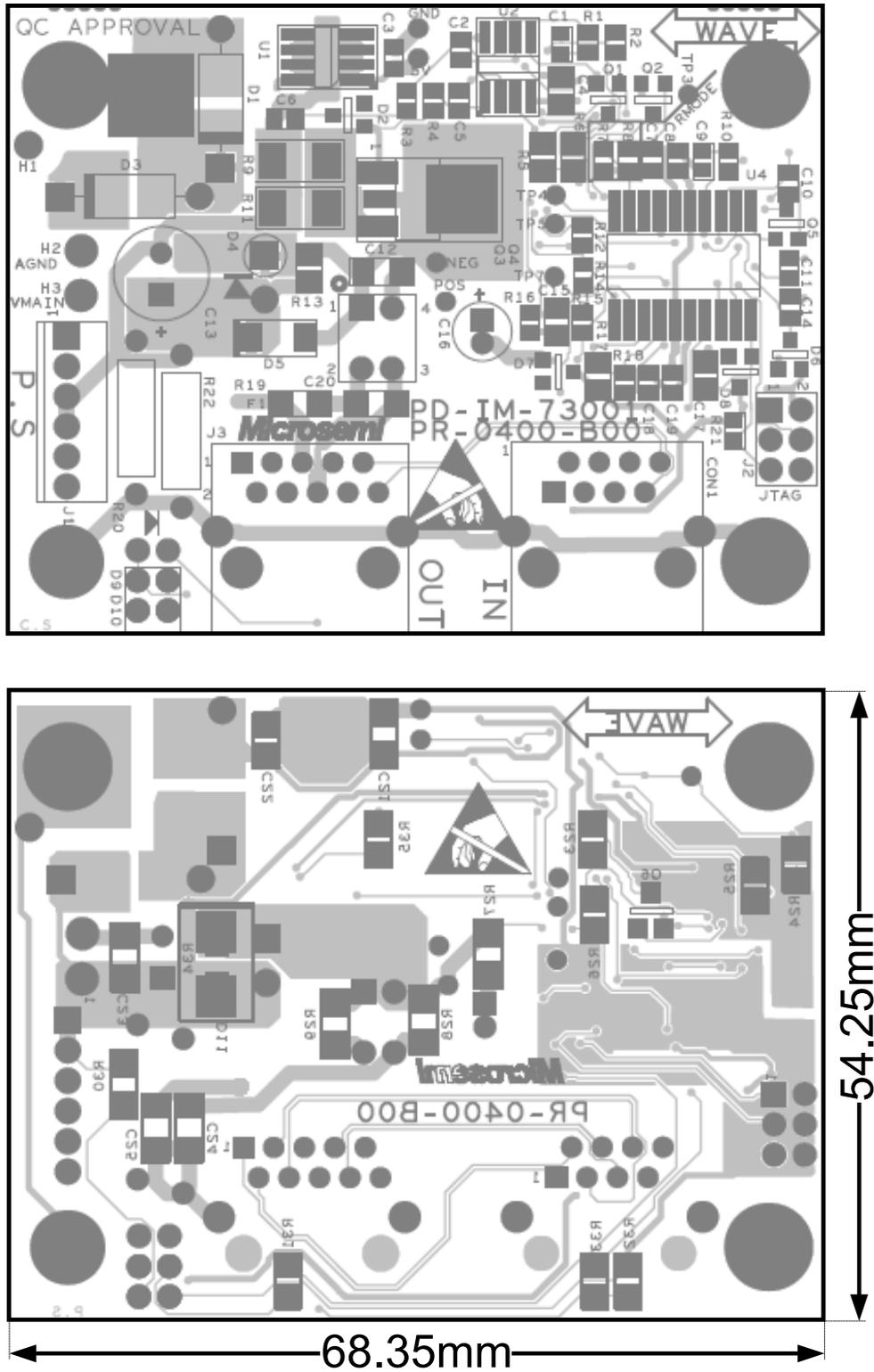
Figure 3: Layout Example of Component and Print Side
