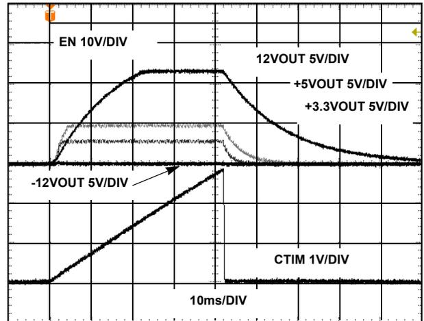
FIGURE 15. ISL6111 TURN-ON INTO M12V OC CONDITION
