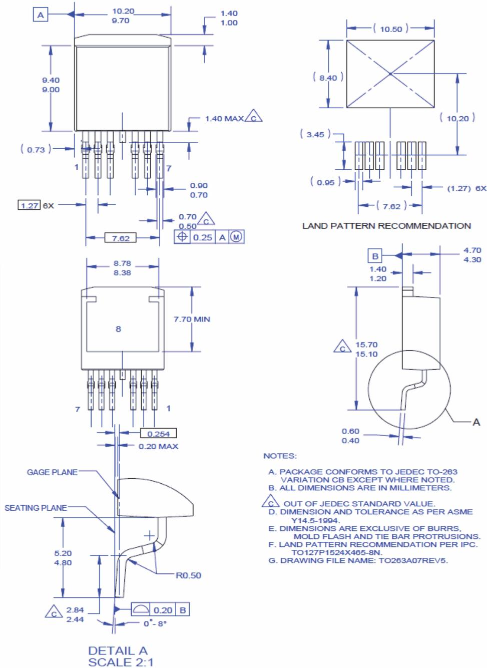
**Figure 17. TO263 (D<sup>2</sup>PAK), Molded, 7-Lead, Surface Mount**
