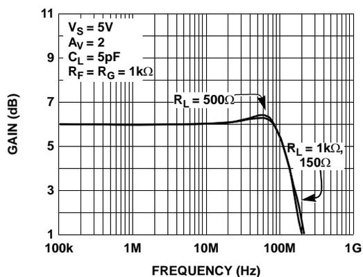
FIGURE 6. SMALL SIGNAL FREQUENCY RESPONSE vs VARIOUS  $R_{LOAD}$
