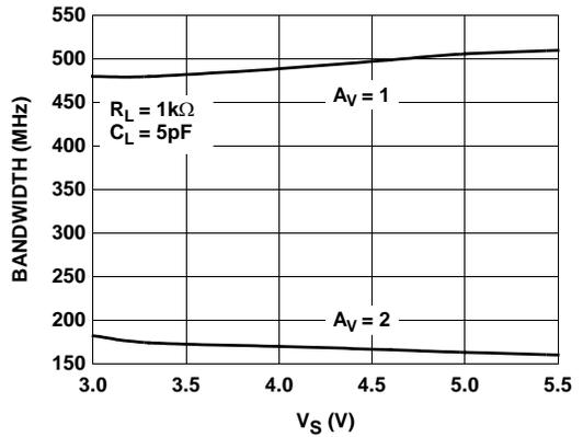
FIGURE 12. SMALL SIGNAL BANDWIDTH vs SUPPLY VOLTAGE
