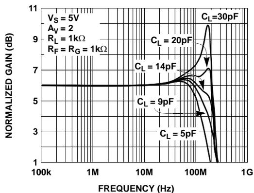
FIGURE 8. SMALL SIGNAL FREQUENCY RESPONSE FOR VARIOUS  $C_L$
