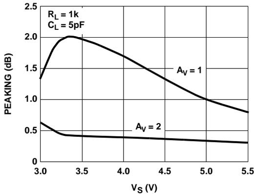
FIGURE 14. SMALL SIGNAL PEAKING vs SUPPLY VOLTAGE
