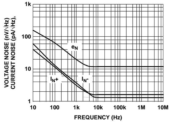
FIGURE 20. VOLTAGE AND CURRENT NOISE vs FREQUENCY
