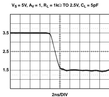
FIGURE 22. LARGE SIGNAL TRANSIENT RESPONSE - FALLING
