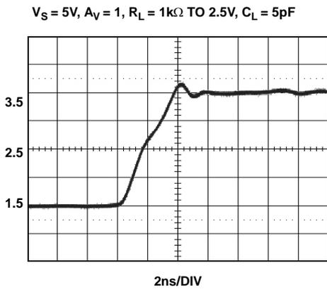
FIGURE 21. LARGE SIGNAL TRANSIENT RESPONSE - RISING
