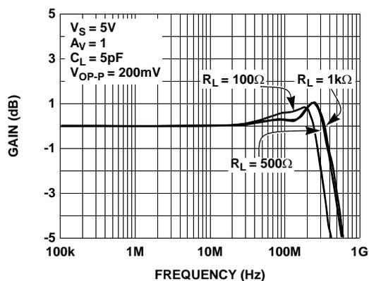
FIGURE 5. SMALL SIGNAL FREQUENCY RESPONSE FOR VARIOUS  $R_{LOAD}$
