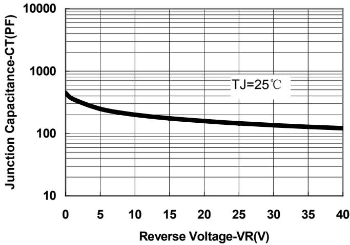
Fig.1-Typical Junction Capacitance
