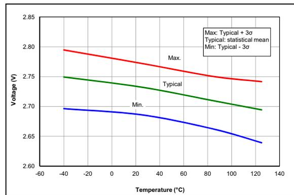
**FIGURE 36-59:** Brown-Out Reset Voltage, High Trip Point ( $BORV = 0$ ).
