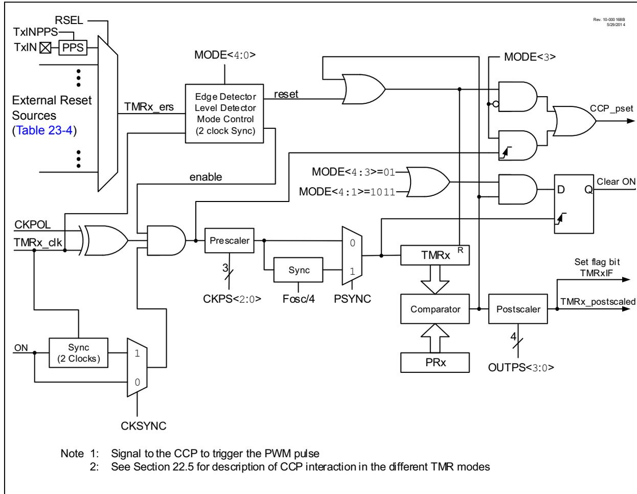
**FIGURE 23-2: TIMER2 CLOCK SOURCE BLOCK DIAGRAM**
