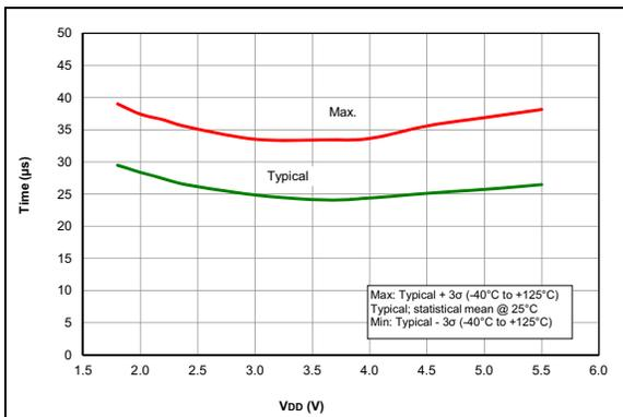
**FIGURE 36-69:** Wake From Sleep,  $V_{REGPM} = 1$ .
