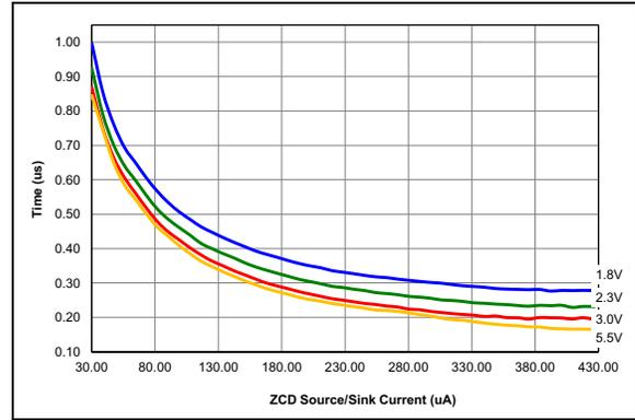
**FIGURE 36-110:** ZCD Pin Response Time over Current, Typical Measured Values from  $-40^\circ C$  to  $125^\circ C$ .
