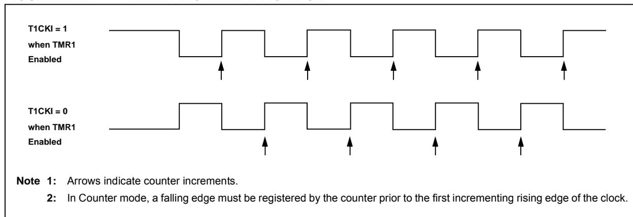
FIGURE 22-3: TIMER1 GATE ENABLE MODE
