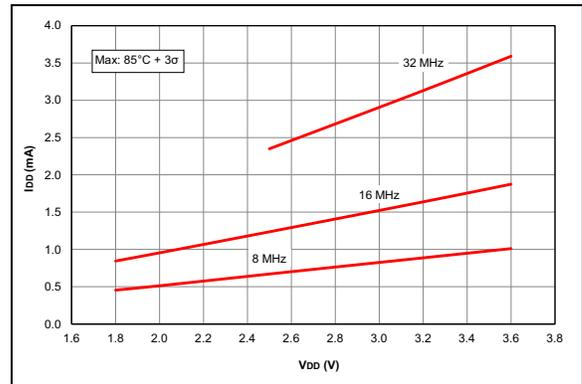
**FIGURE 36-18:**  $I_{DD}$  Maximum, HFINTOSC Mode, PIC16LF1615/9 Only.
