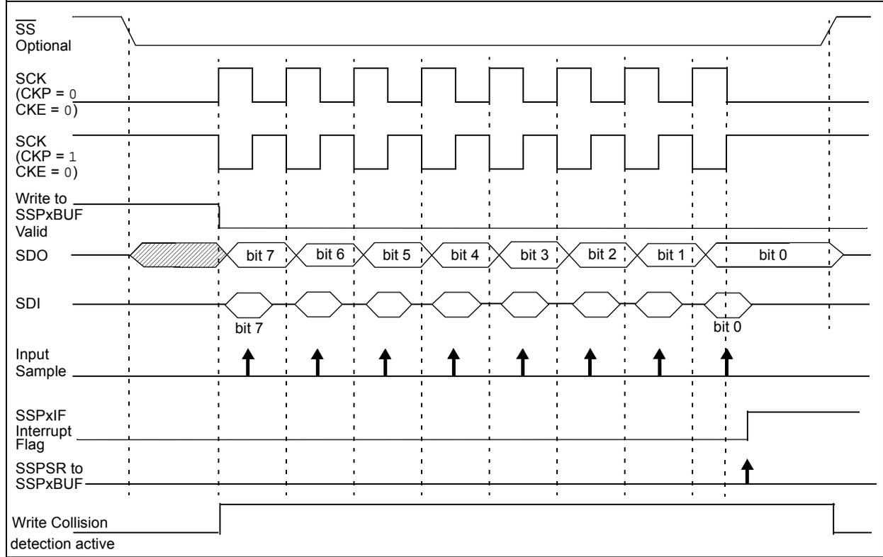
**FIGURE 24-10: SPI MODE WAVEFORM (SLAVE MODE WITH CKE = 1)**
