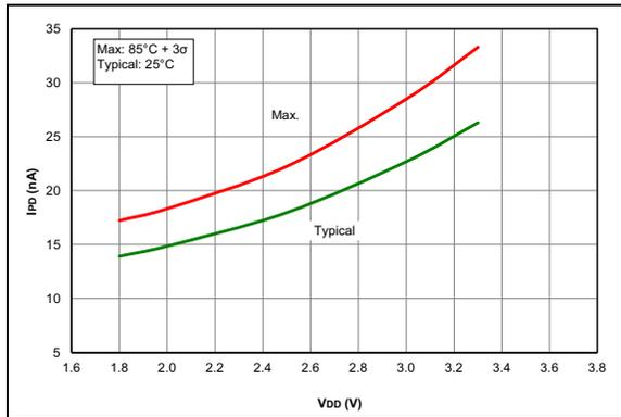
**FIGURE 36-31:**  $I_{PD}$ , Fixed Voltage Reference (FVR), PIC16LF1615/9 Only.
