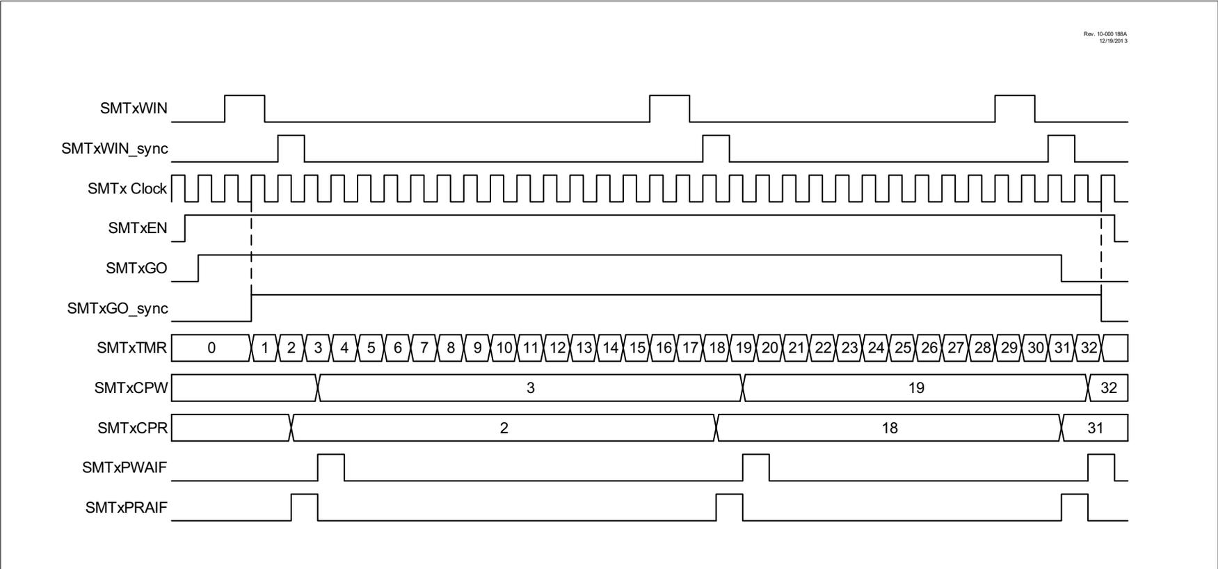
**FIGURE 30-17: CAPTURE MODE SINGLE ACQUISITION TIMING DIAGRAM**
