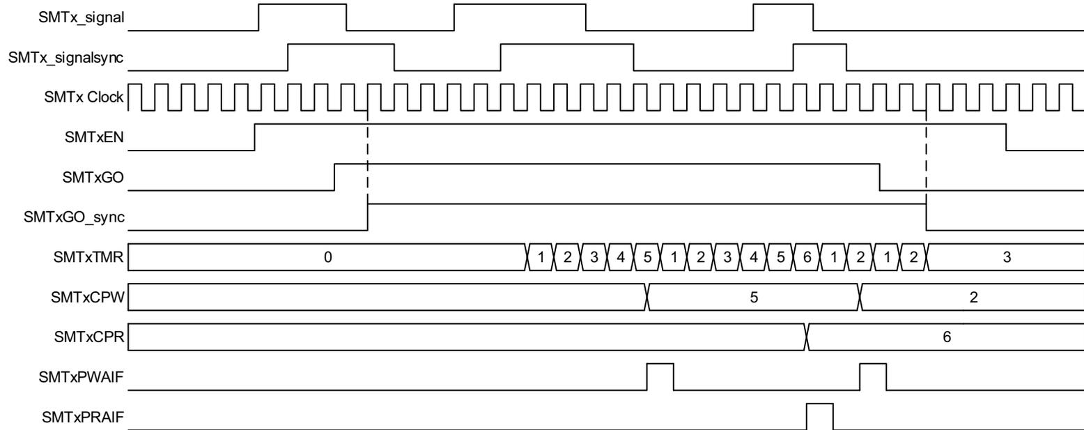
**FIGURE 30-9: HIGH AND LOW MEASURE MODE SINGLE ACQUISITION TIMING DIAGRAM**
