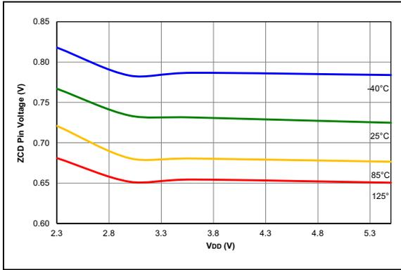
**FIGURE 36-107:** ZCD Pin Voltage, Typical Measured Values.
