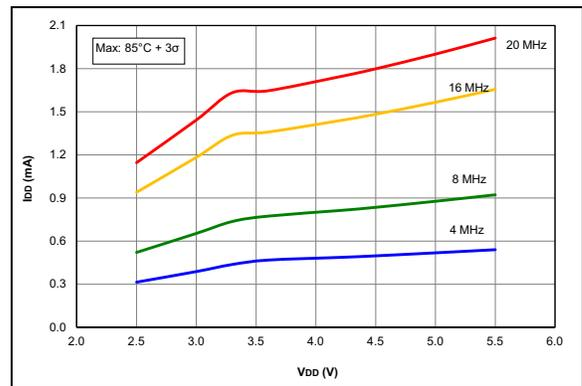
**FIGURE 36-24:**  $I_{DD}$  Maximum, HS Oscillator, PIC16F1615/9 Only.
