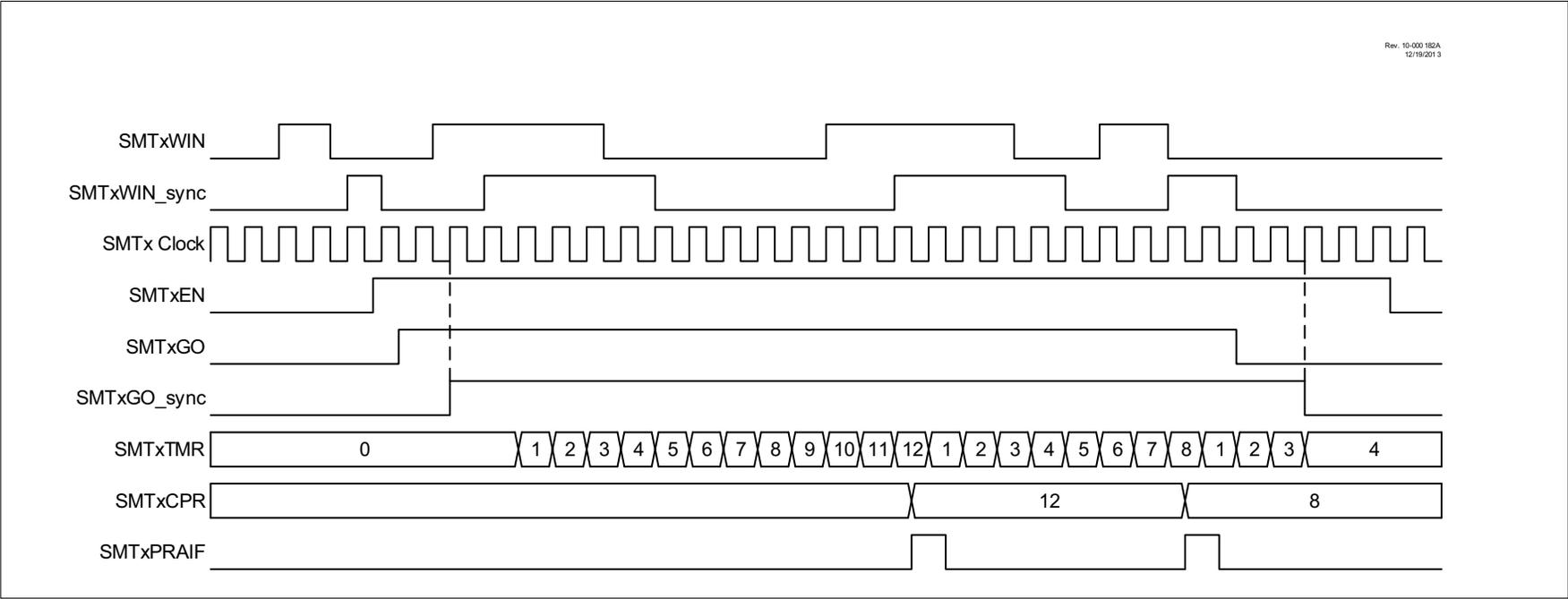
**FIGURE 30-11: WINDOWED MEASURE MODE SINGLE ACQUISITION TIMING DIAGRAM**
