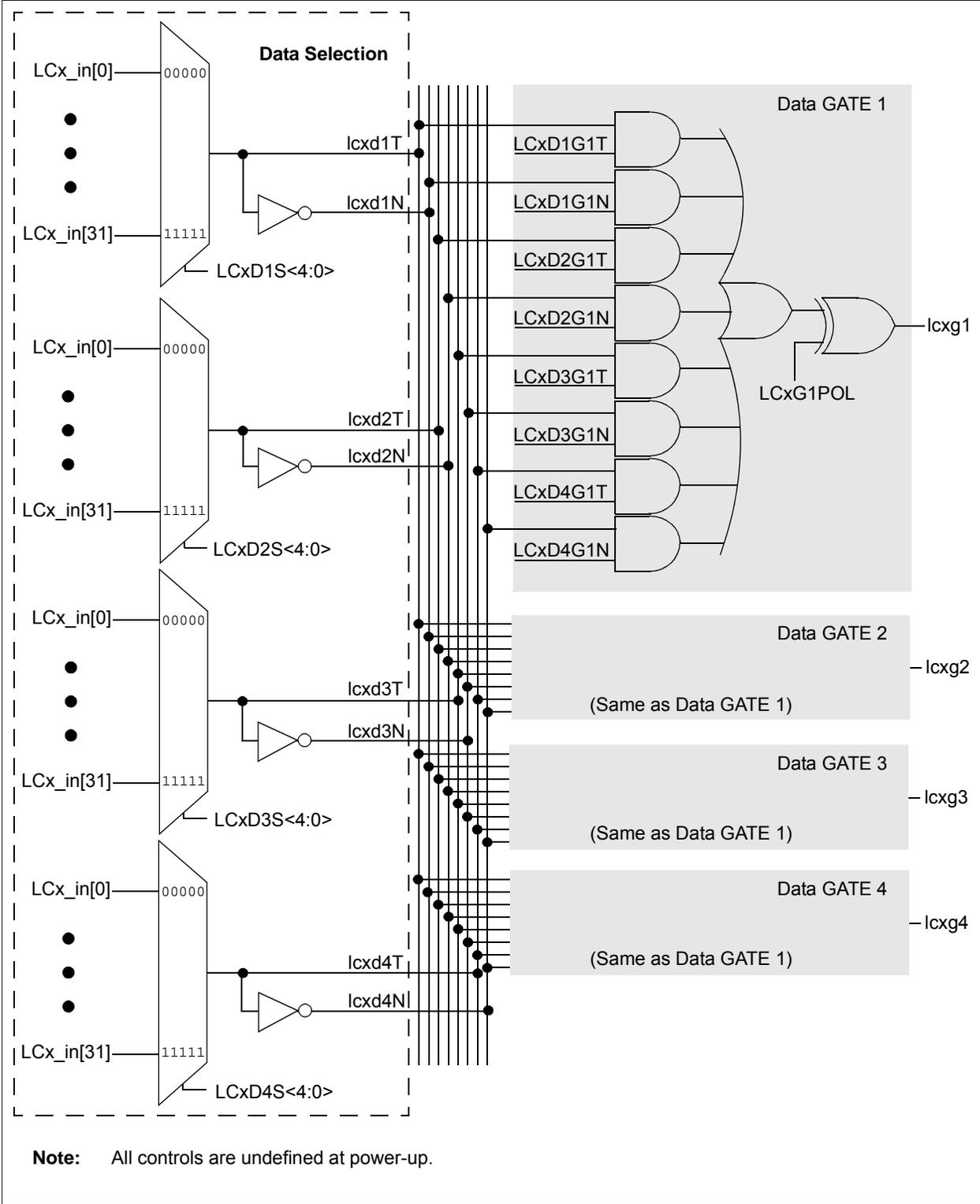
FIGURE 29-3: PROGRAMMABLE LOGIC FUNCTIONS
