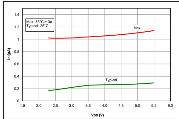
**FIGURE 36-40:**  $I_{PD}$ , ADC Non-Converting, PIC16F1615/9 Only.
