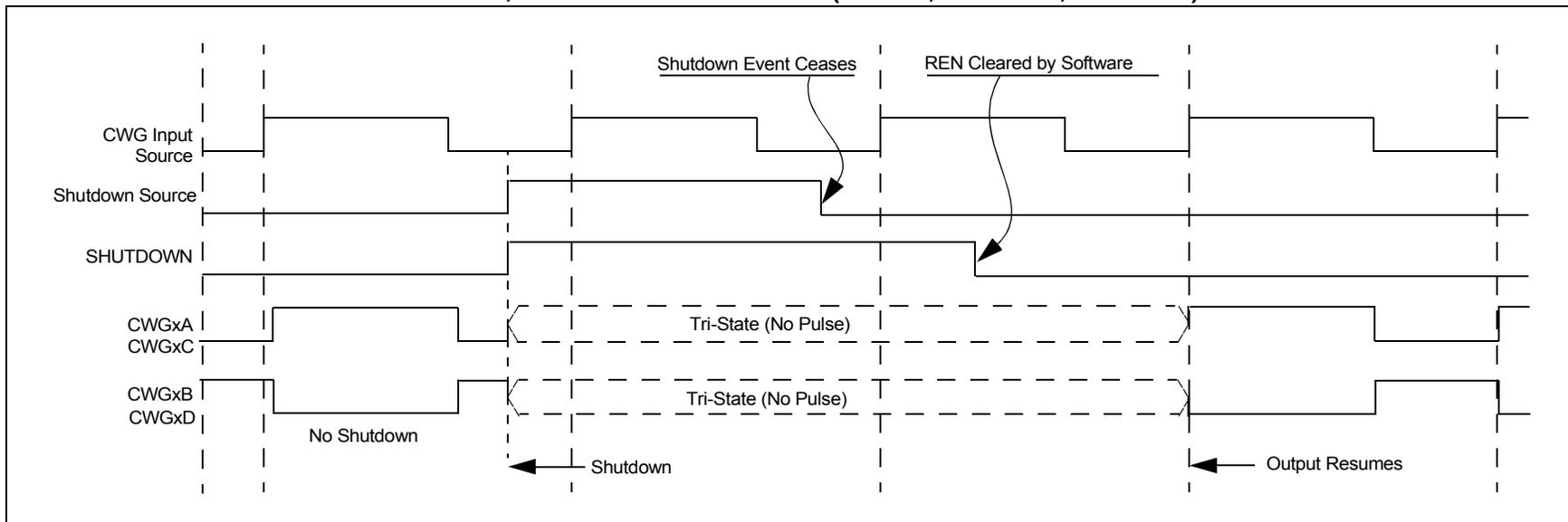
**FIGURE 28-14: SHUTDOWN FUNCTIONALITY, AUTO-RESTART ENABLED (REN = 1, LSAC = 01, LSB0 = 01)**
