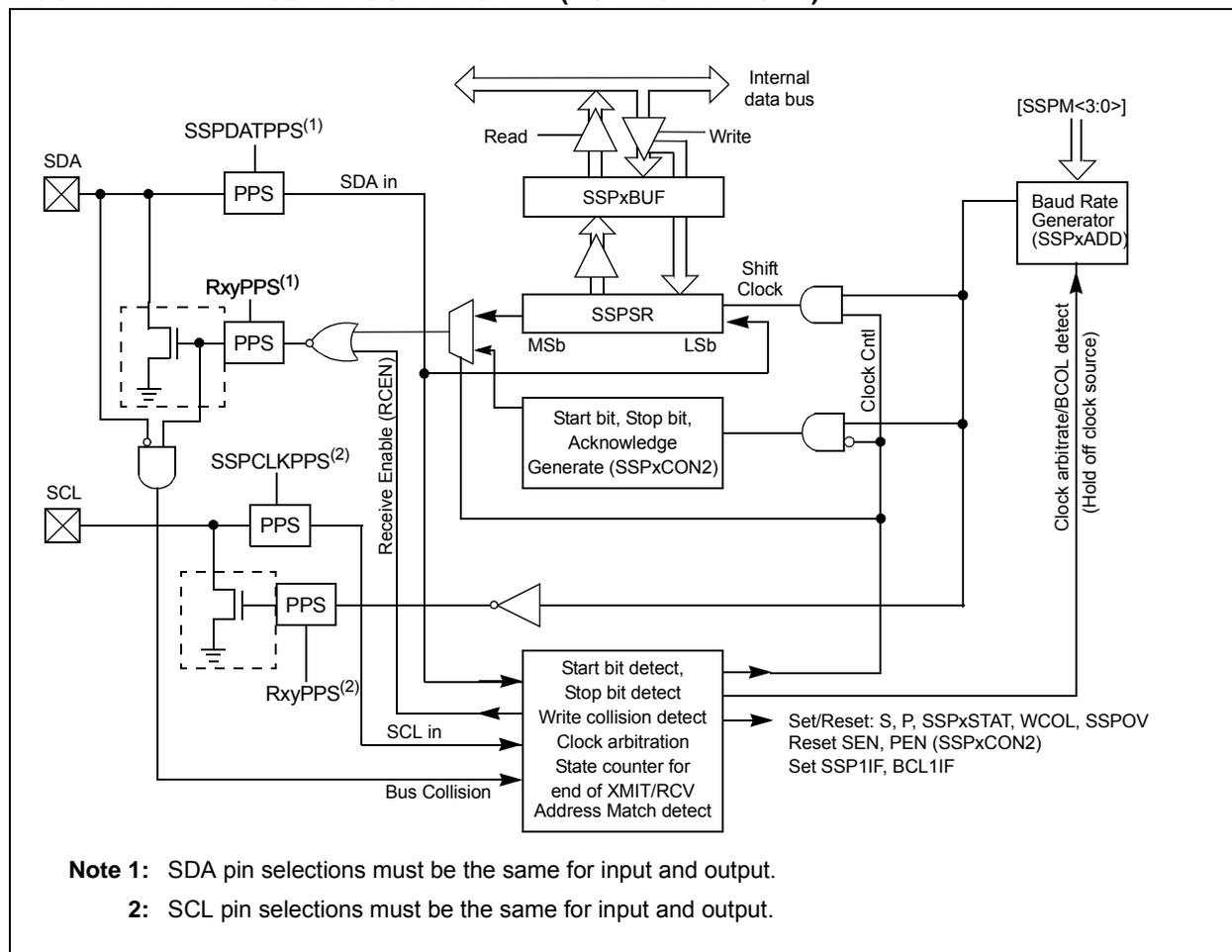
FIGURE 24-3: MSSP BLOCK DIAGRAM (I<sup>2</sup>C SLAVE MODE)
