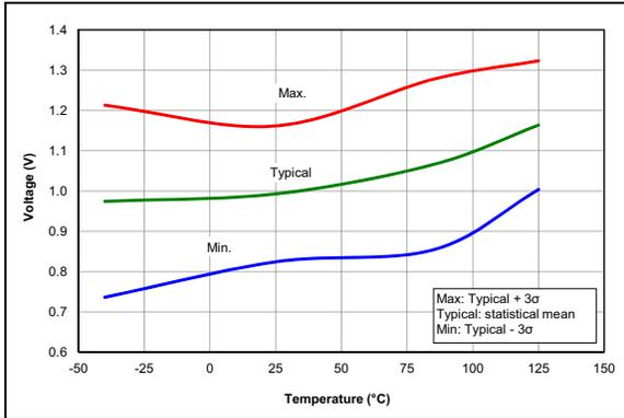
**FIGURE 36-67:** POR Rearm Voltage, NP Mode, PIC16LF1615/9 Only.
