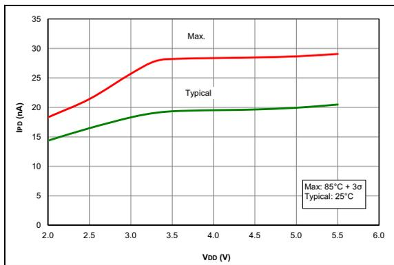
**FIGURE 36-32:**  $I_{PD}$ , Fixed Voltage Reference (FVR), PIC16F1615/9 Only.
