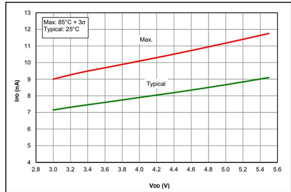
**FIGURE 36-34:**  $I_{PD}$ , Brown-Out Reset (BOR), BORV = 1, PIC16F1615/9 Only.
