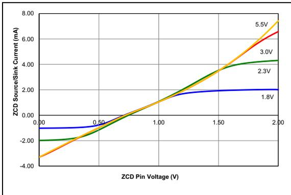
**FIGURE 36-109:** ZCD Pin Current over ZCD Pin Voltage, Typical Measured Values from  $-40^\circ C$  to  $125^\circ C$ .
