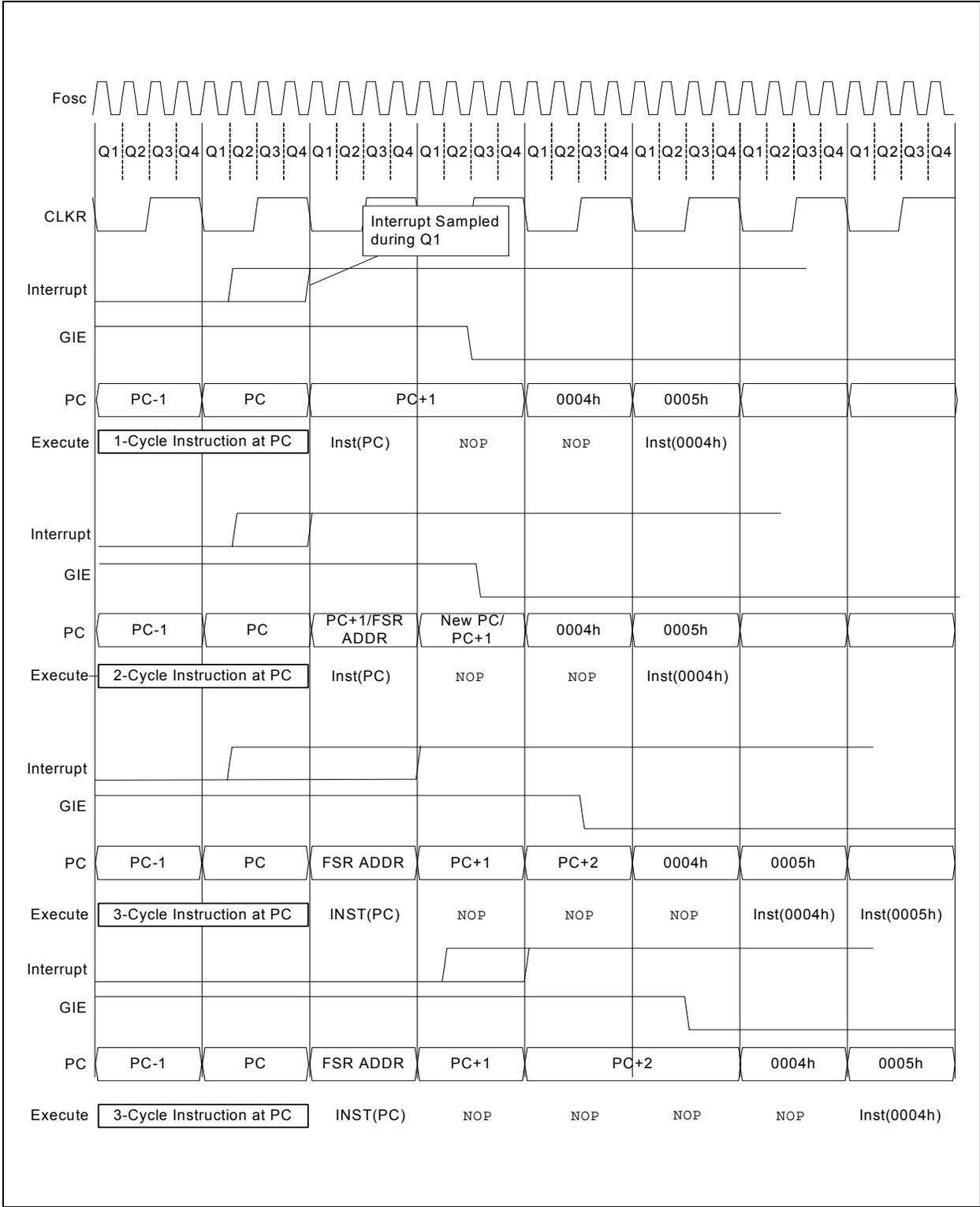
**FIGURE 7-3: INT PIN INTERRUPT TIMING**
