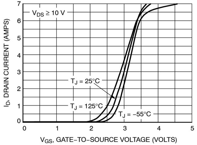
**Figure 2. Transfer Characteristics**
