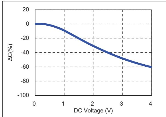
4) Bias TCC characteristics (Agilent 4284A, 1kHz, 0.5Vrms, 2Vdc)
