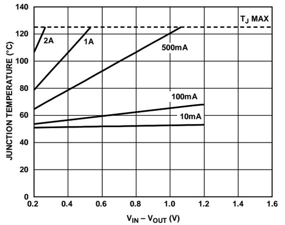
Figure 39. 25 mm<sup>2</sup> of PCB Copper,  $T_A = 50^\circ\text{C}$
