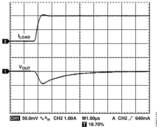
Figure 31. Output Transient Response,  $C_{OUT} = 10 \mu\text{F}$
