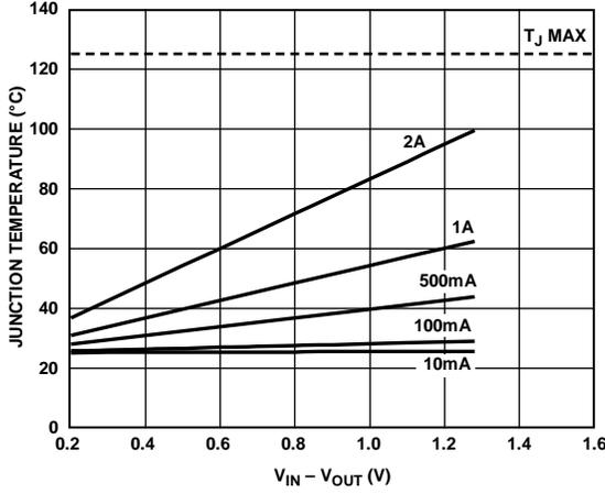
Figure 40. 500 mm<sup>2</sup> of PCB Copper,  $T_B = 25^\circ\text{C}$
