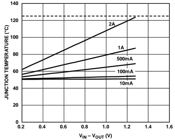
Figure 43. 1000 mm<sup>2</sup> of PCB Copper,  $T_B = 50^\circ\text{C}$
