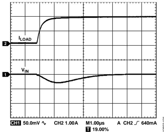
Figure 32. Output Transient Response,  $C_{OUT} = 47 \mu\text{F}$
