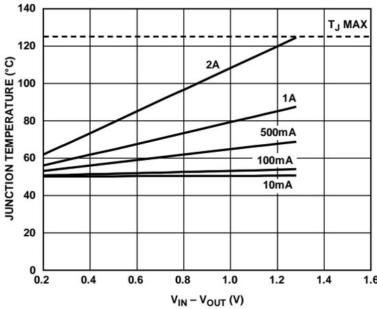
Figure 41. 500 mm<sup>2</sup> of PCB Copper,  $T_B = 50^\circ\text{C}$
