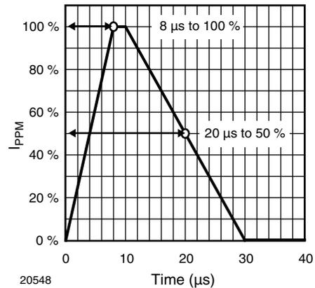
Fig. 2 - 8/20  $\mu\text{s}$  Peak Pulse Current Wave Form
