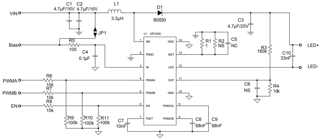
**Figure 2—Typical Application Driving 9 Strings of 3 WLEDs**
