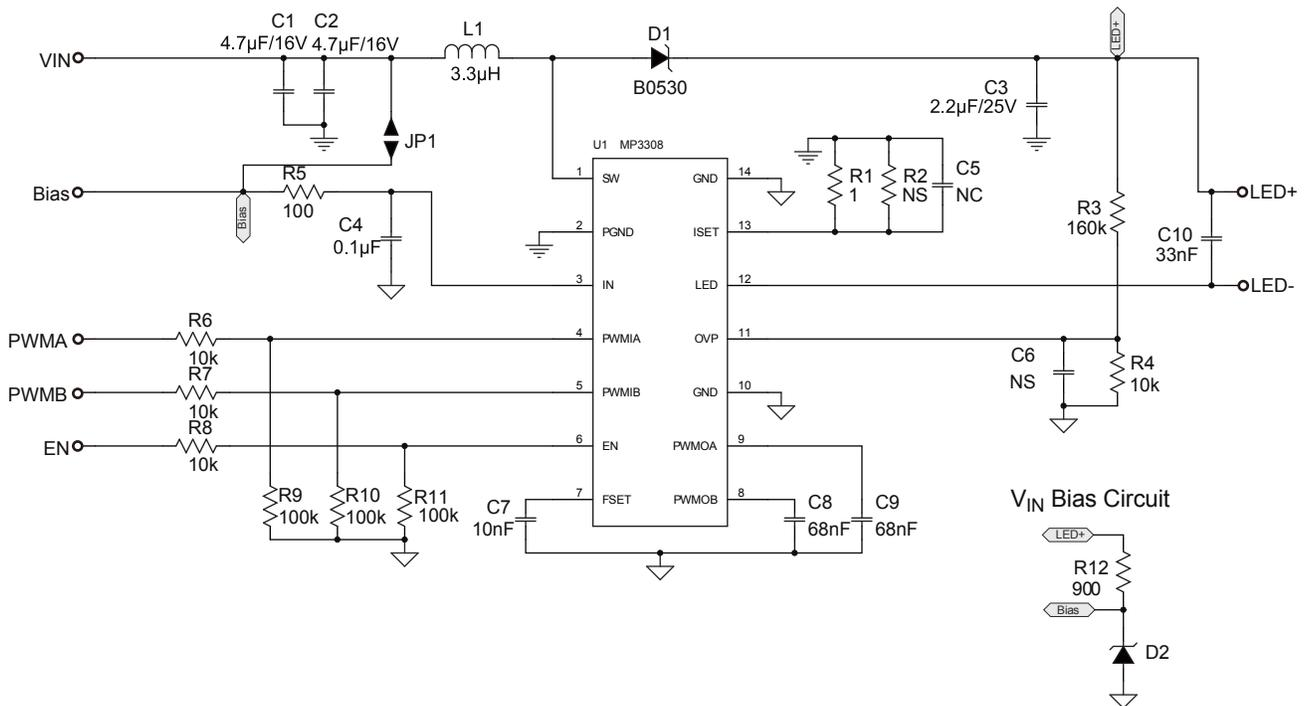
**Figure 4— Driving 27 WLEDs (9 WLEDs in Series and 3 Strings Paralleled) with 3V-3.3V Input Voltage<sup>1</sup>**
