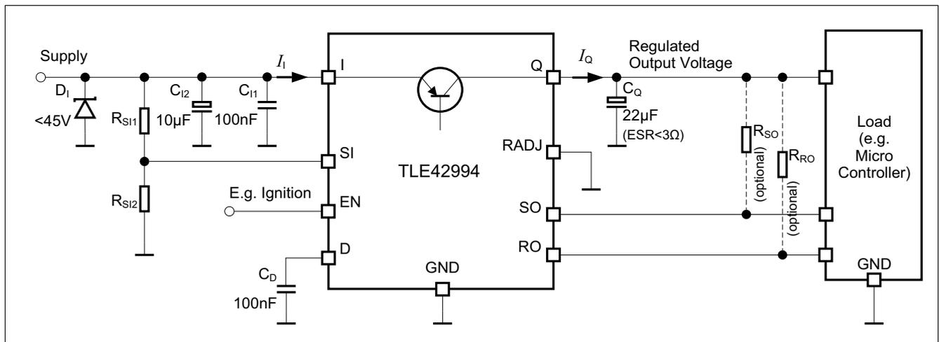
Figure 8 Application Diagram with Selecting Default Reset Thresholds
