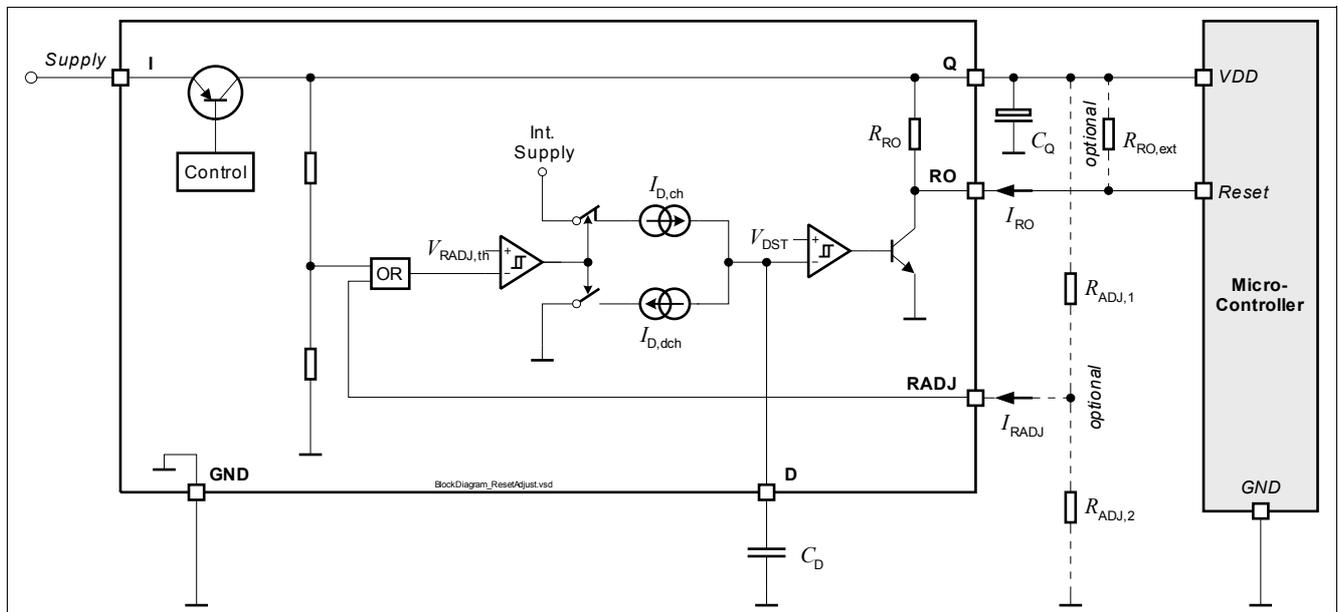
Figure 5 Block Diagram Reset Function
