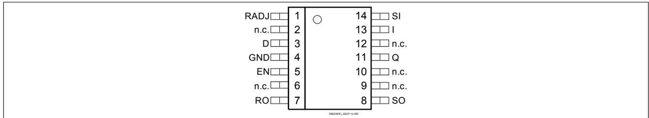
Figure 3 Pin Configuration (top view)
