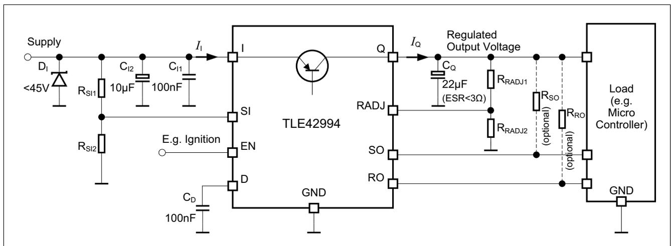
Figure 9 Application Diagram with Reset Thresholds Adjustment
