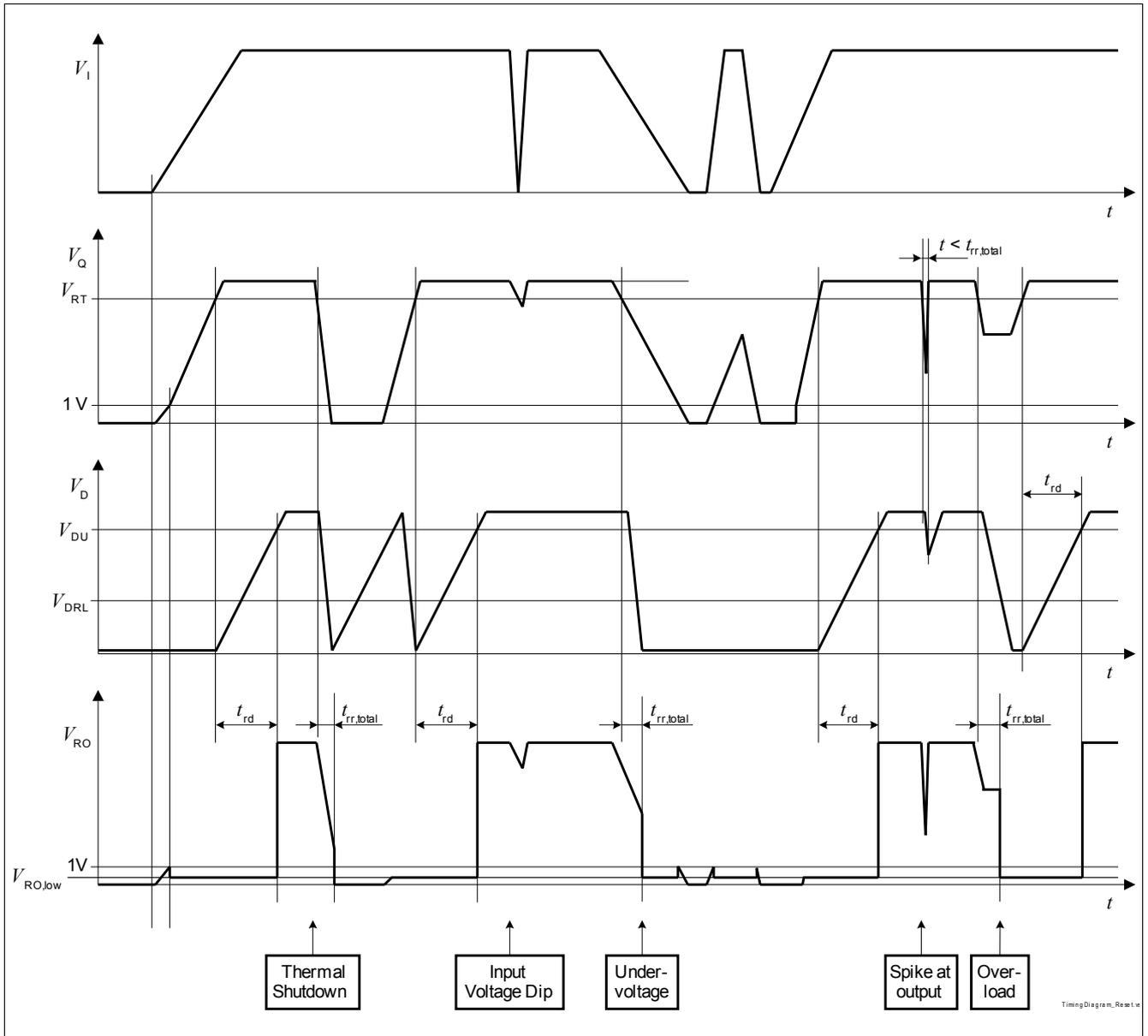
Figure 6 Timing Diagram Reset
