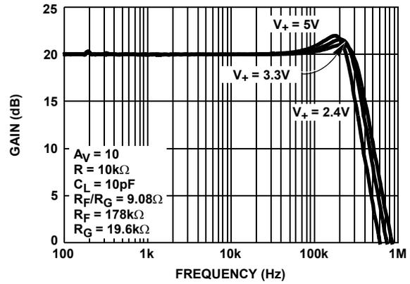
FIGURE 8. ISL28273 FREQUENCY RESPONSE vs SUPPLY VOLTAGE
