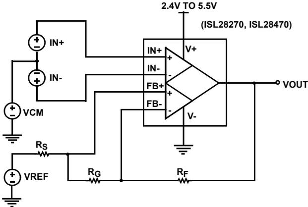
FIGURE 51. REFERENCE CONNECTION WITH AN AVAILABLE VREF
