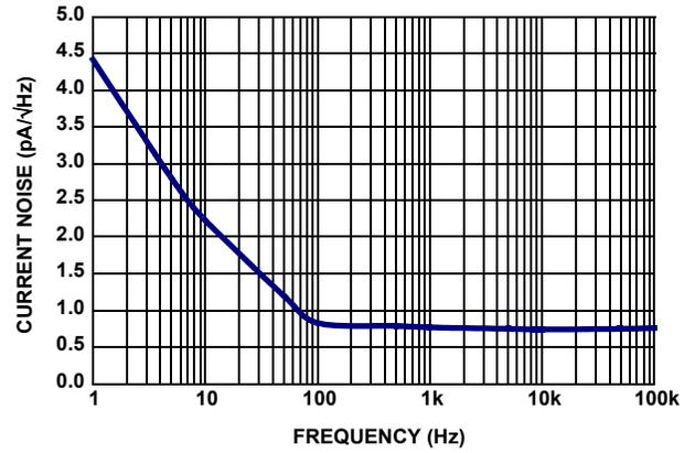
FIGURE 18. ISL28273 INPUT CURRENT NOISE SPECTRAL DENSITY (GAIN = 10)
