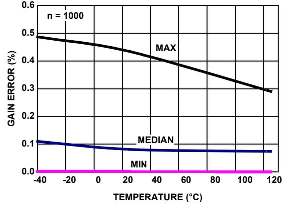
FIGURE 44. ISL28273 % GAIN ERROR vs TEMPERATURE,  $R_L = 100k$
