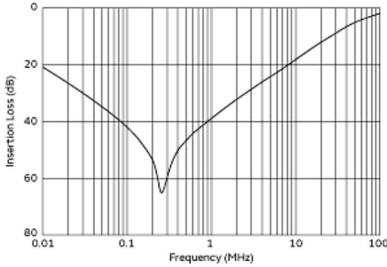
Common Mode Insertion Loss (Typ.)
