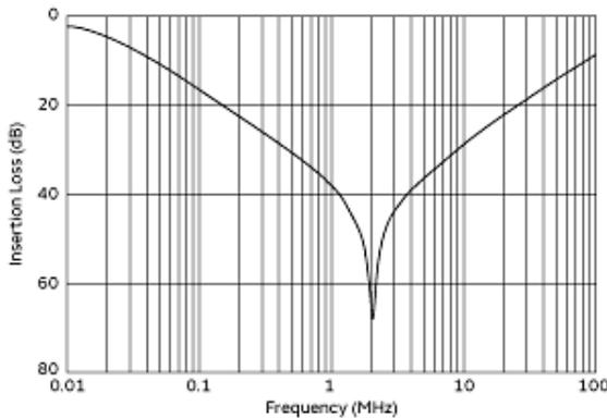
Differential Mode Insertion Loss (Typ.)
