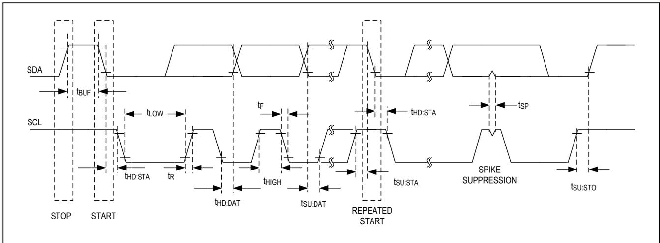
Figure 43: I<sup>2</sup>C Timing Diagram
