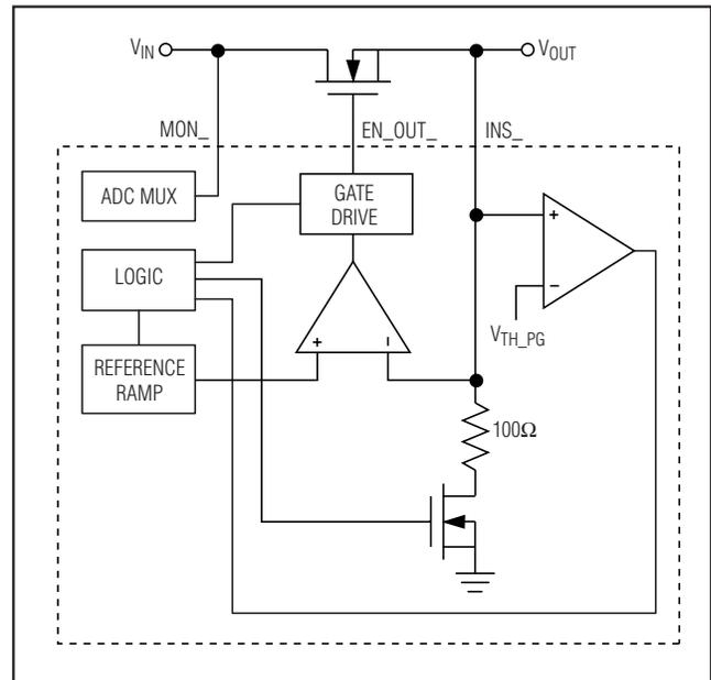
Figure 19. Closed-Loop Tracking
