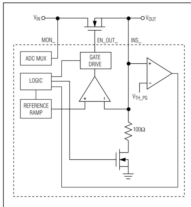
Figure 5. Closed-Loop Tracking
