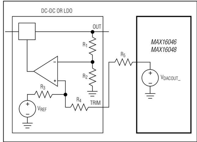
Figure 17. Connections for Margining Using Trim Input Method
