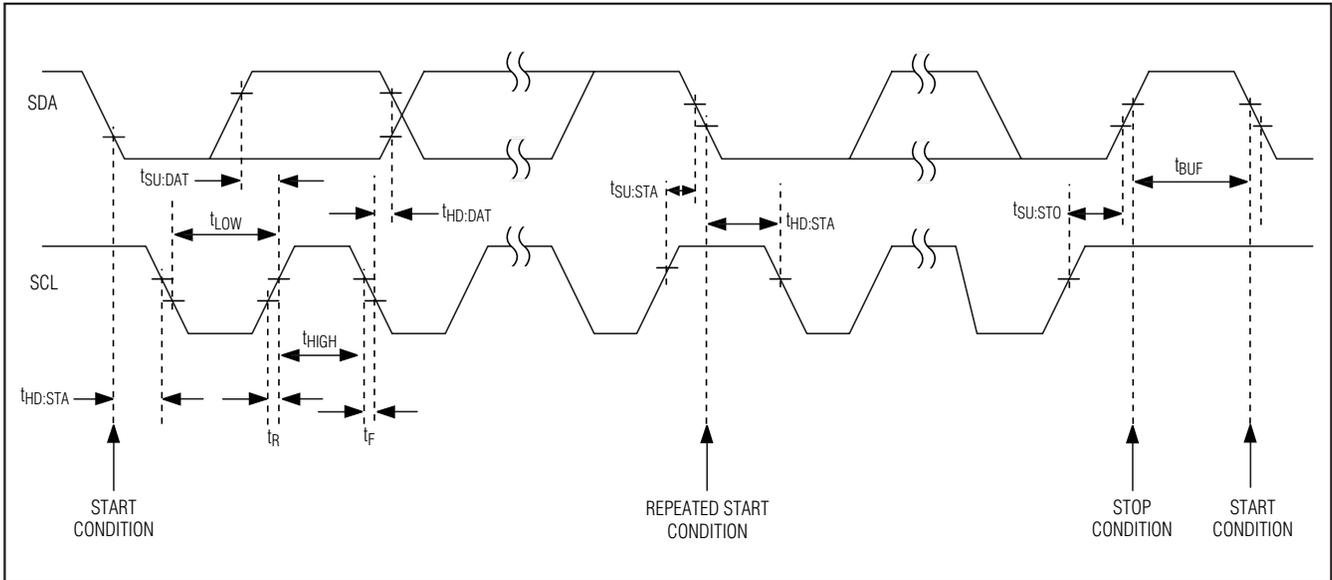
Figure 1. I<sup>2</sup>C/SMBus Timing Diagram
