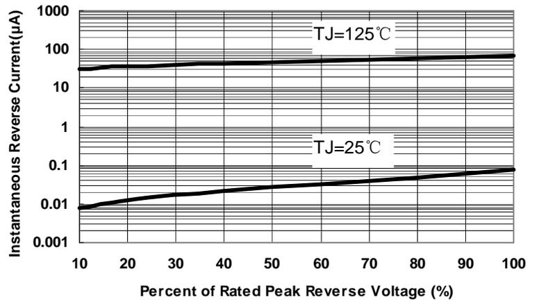
Fig.2-Typical Reverse Characteristics
