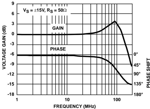
FIGURE 4. GAIN/PHASE vs FREQUENCY ( $R_L = 1k\Omega$ )
