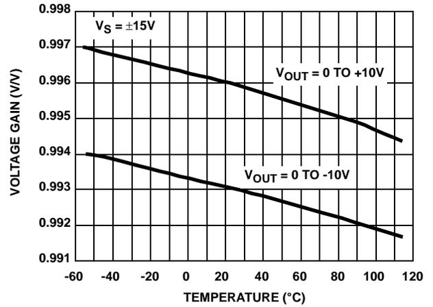
FIGURE 7. VOLTAGE GAIN vs TEMPERATURE ( $R_L = 1k\Omega$ )
