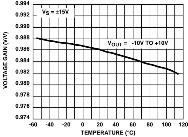
FIGURE 6. VOLTAGE GAIN vs TEMPERATURE ( $R_L = 100\Omega$ )
