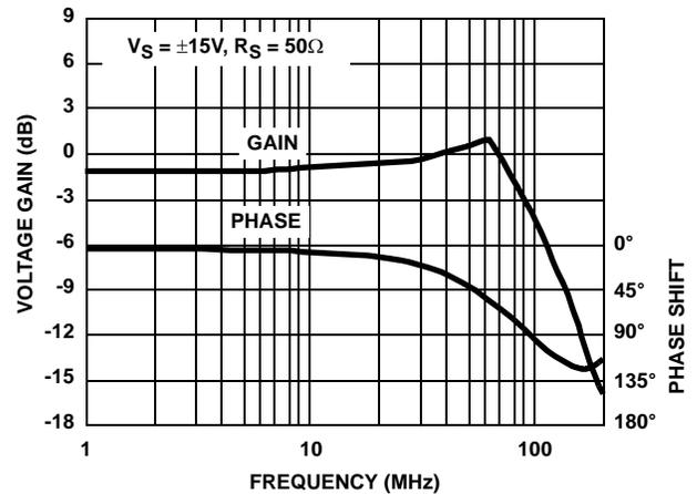
FIGURE 5. GAIN/PHASE vs FREQUENCY ( $R_L = 50\Omega$ )
