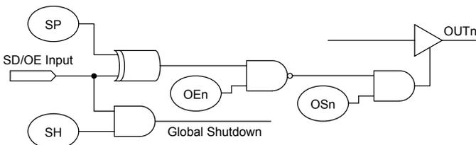
When configured as SD, device is shut down, differential
