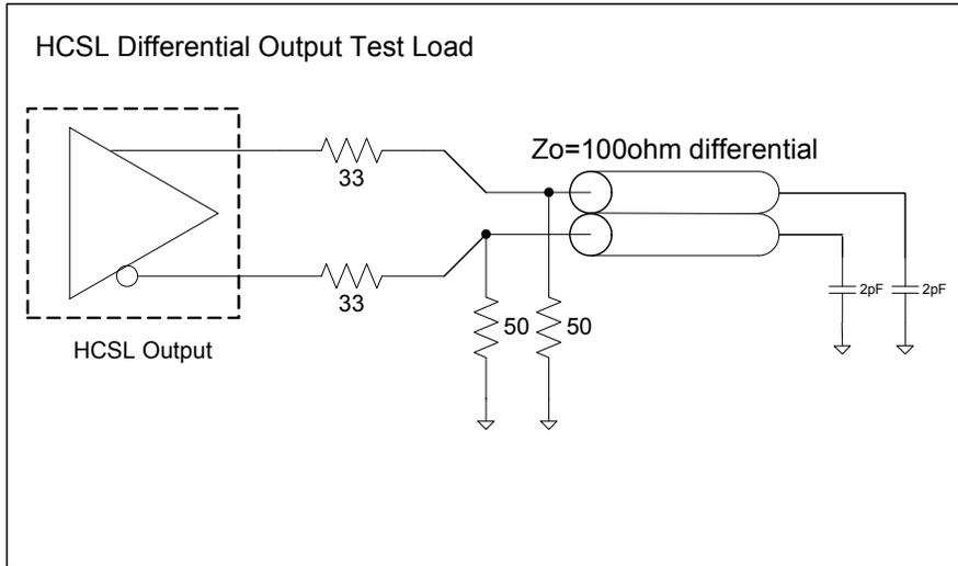
**Test Circuits and Loads for Outputs**
