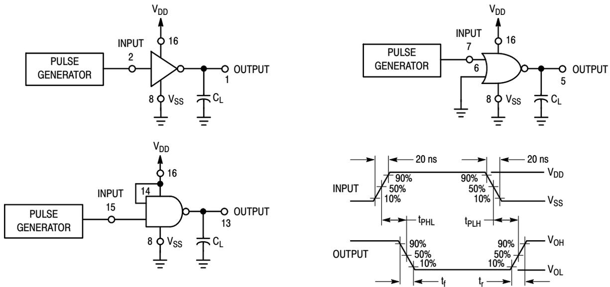
Figure 1. Switching Time Test Circuits and Waveforms
