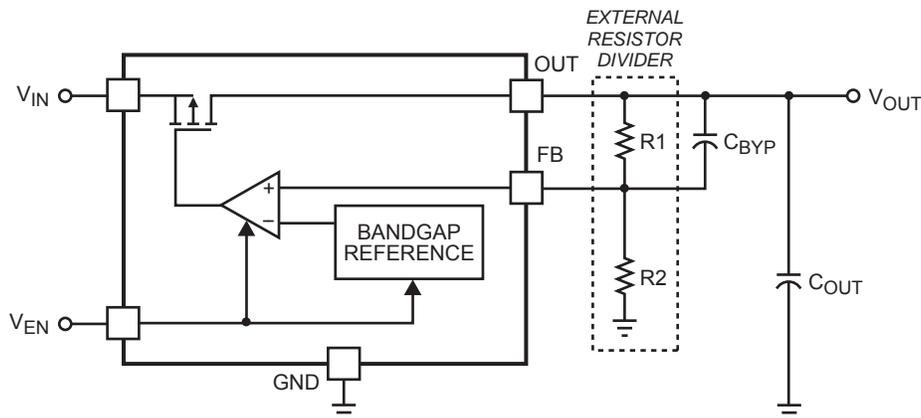
**Figure 2—Adjustable Regulator:  $V_{OUT} = V_{FB} (1 + (R1/R2))$**
