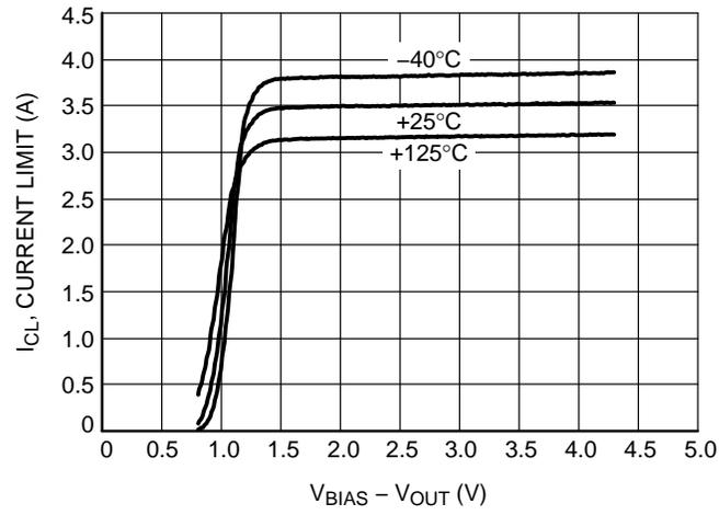
Figure 15. Current Limit vs. ( $V_{BIAS} - V_{OUT}$ )
