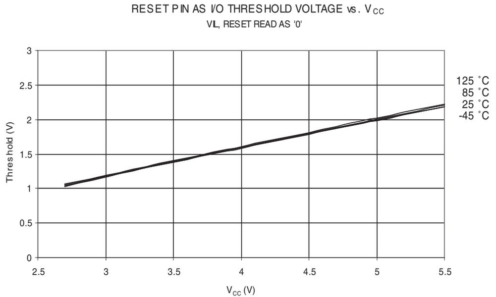
**Figure 23-28.** Reset Pin Input Hysteresis vs.  $V_{CC}$
