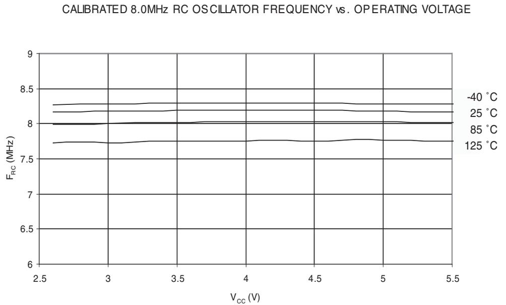
**Figure 23-34.** Calibrated 8MHz RC oscillator Frequency vs. Temperature
