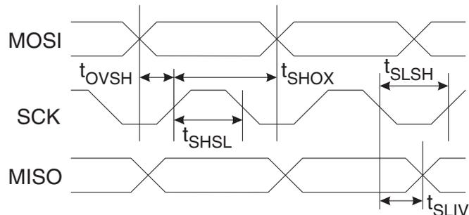
**Figure 22-4.** Serial Programming Waveforms
