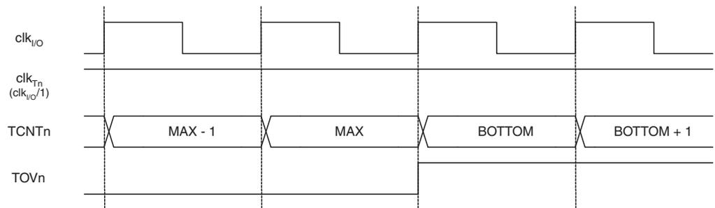
[Figure 13-9 on page 82](#) shows the same timing data, but with the prescaler enabled.
