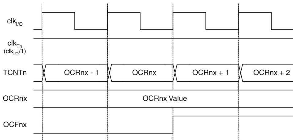
[Figure 14-11 on page 111](#) shows the same timing data, but with the prescaler enabled.
