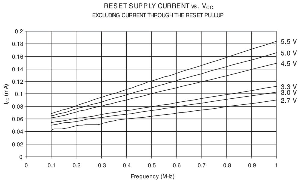
**Figure 23-42.** Reset Supply Current vs.  $V_{CC}$  (1 - 20MHz, Excluding Current Through the Reset Pull-up)
