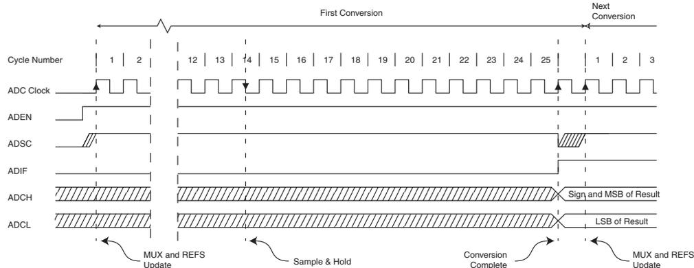
**Figure 18-5.** ADC Timing Diagram, Single Conversion
