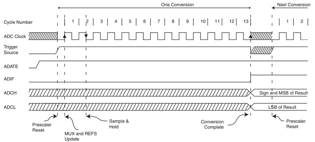
**Figure 18-7.** ADC Timing Diagram, Free Running Conversion
