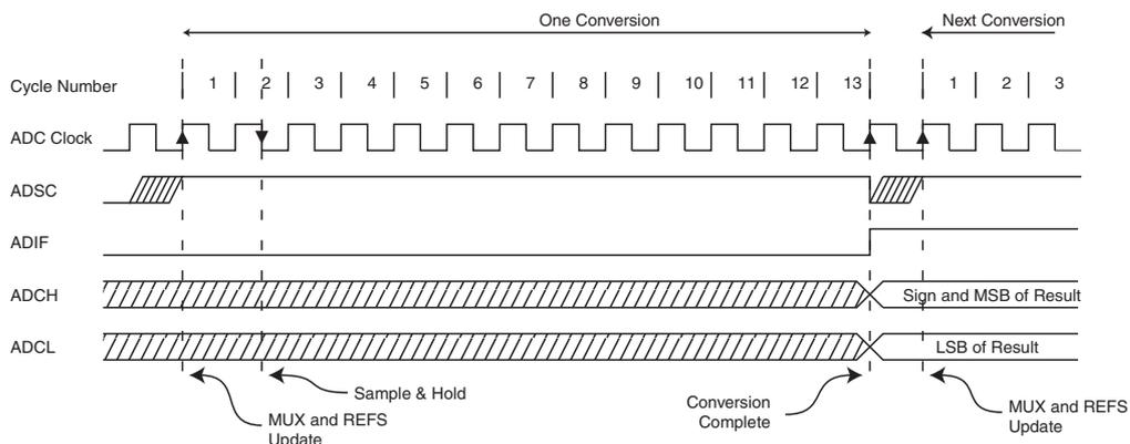
**Figure 18-6.** ADC Timing Diagram, Auto Triggered Conversion
