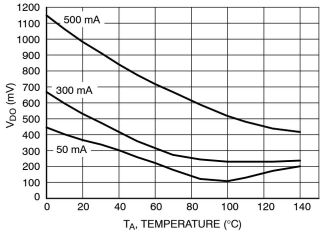
**Figure 14. Dropout Voltage vs. Temperature
