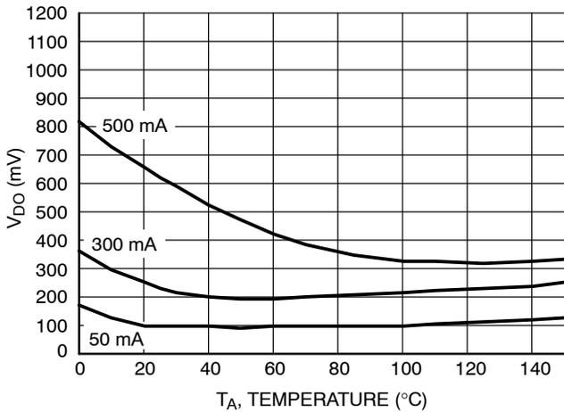
**Figure 13. Dropout Voltage vs. Temperature
