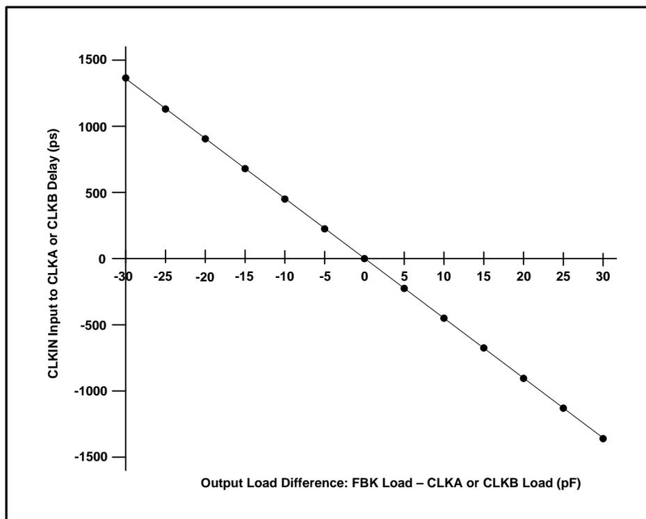
Figure 1. CLKIN Input to CLK A and B Delay
