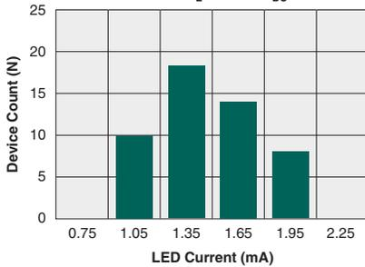
**Typical I<sub>F</sub> for Switch Dropout**
