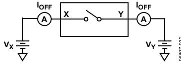
Figure 26. Off Leakage
