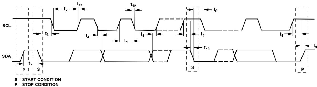
Figure 2. Timing Diagram for 2-Wire Serial Interface
