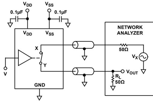
$$\text{INSERTION LOSS} = 20 \log \frac{V_{OUT} \text{ WITH SWITCH}}{V_{OUT} \text{ WITHOUT SWITCH}}$$
