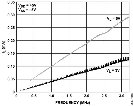
Figure 22. Digital Current ( $I_L$ ) vs. Frequency
