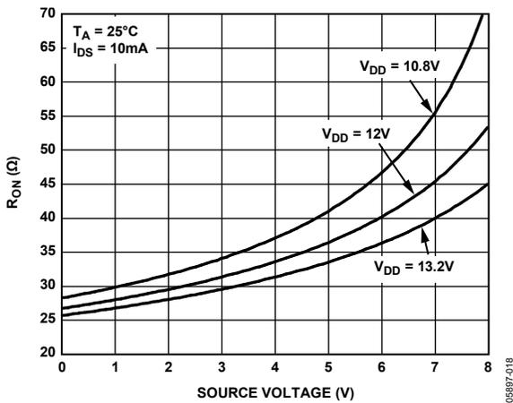
Figure 6.  $R_{ON}$  vs. Supplies,  $V_{DD} = 12\text{V} \pm 10\%$
