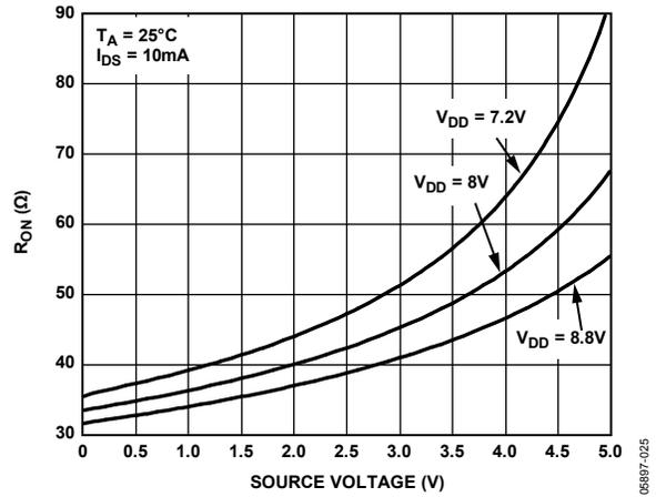
Figure 7.  $R_{ON}$  vs. Source Voltage,  $V_{DD} = 8\text{V} \pm 10\%$
