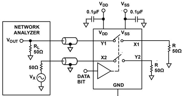
CHANNEL-TO-CHANNEL CROSSTALK =  $20 \log \frac{V_{OUT}}{V_S}$
