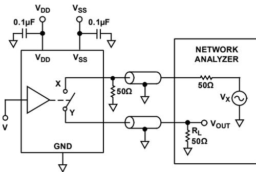
$$\text{OFF ISOLATION} = 20 \log \frac{V_{OUT}}{V_S}$$
