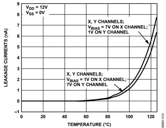
Figure 14. Off Leakage vs. Temperature, 12 V Single Supply
