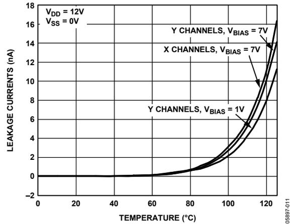
Figure 13. On Leakage vs. Temperature, 12 V Single Supply
