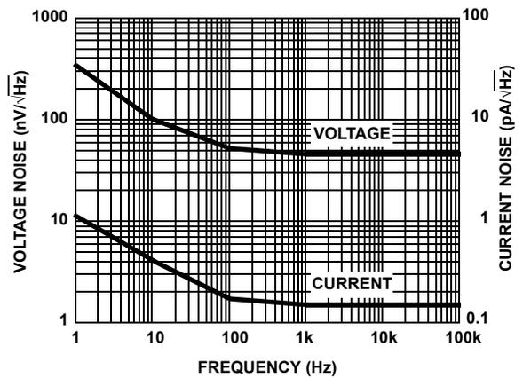
FIGURE 10. INPUT VOLTAGE AND CURRENT NOISE vs FREQUENCY
