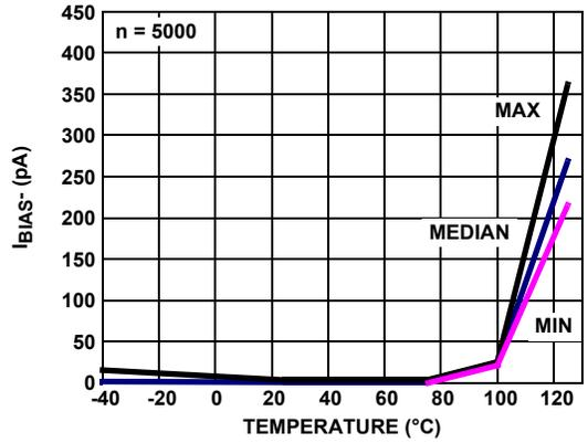
FIGURE 19.  $I_{BIAS-}$  vs TEMPERATURE,  $V_S = \pm 2.5V$
