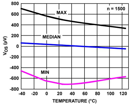
FIGURE 17.  $V_{OS}$  vs TEMPERATURE,  $V_S = \pm 1.2V$
