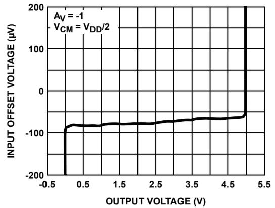
FIGURE 4. INPUT OFFSET VOLTAGE vs OUTPUT VOLTAGE
