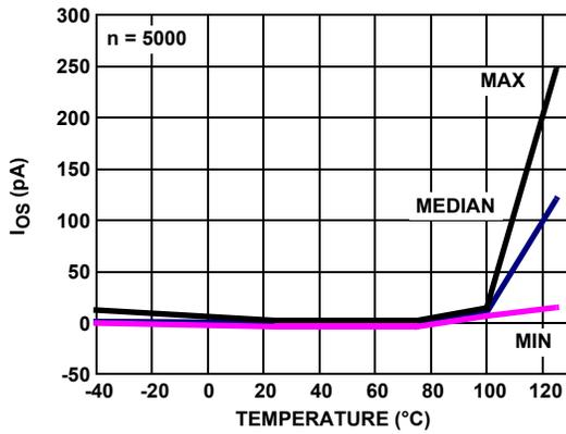
FIGURE 20.  $I_{OS}$  vs TEMPERATURE,  $V_S = \pm 2.5V$
