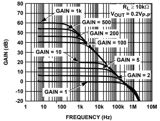
FIGURE 2. FREQUENCY RESPONSE at VARIOUS CLOSED LOOP GAINS
