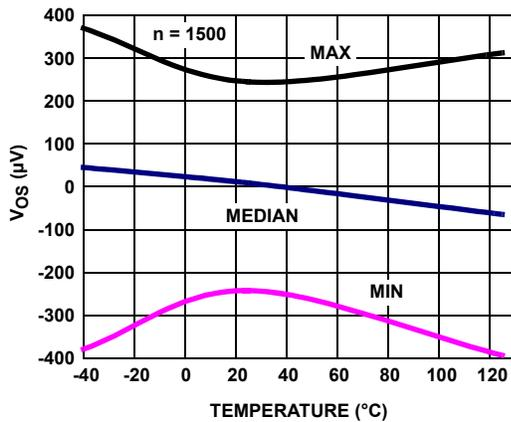
FIGURE 16.  $V_{OS}$  vs TEMPERATURE,  $V_S = \pm 2.5V$
