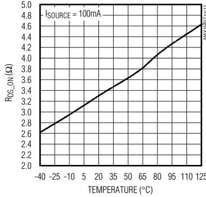
**OUT IMPEDANCE vs. TEMPERATURE (R<sub>DS\_ON</sub> NMOS DRIVER)**
