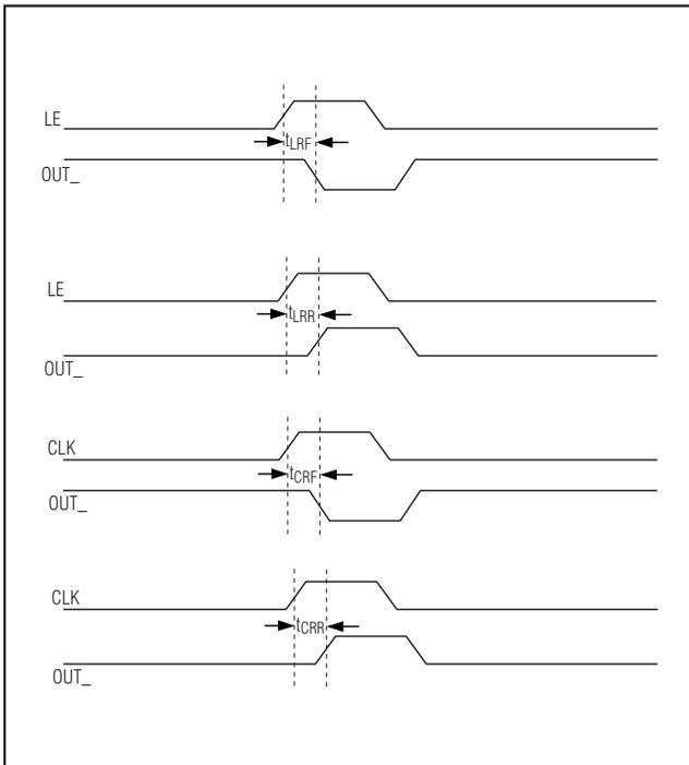
Figure 4. LE and CLK to OUT\_ Timing
