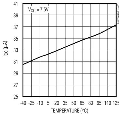
**OPERATING SUPPLY CURRENT vs. TEMPERATURE AFTER STARTUP**
