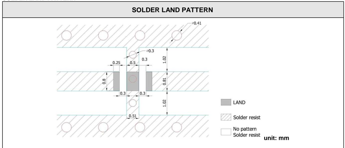
Line width to be designed to match 50 Ω characteristic impedance, depending on PCB material and thickness.
