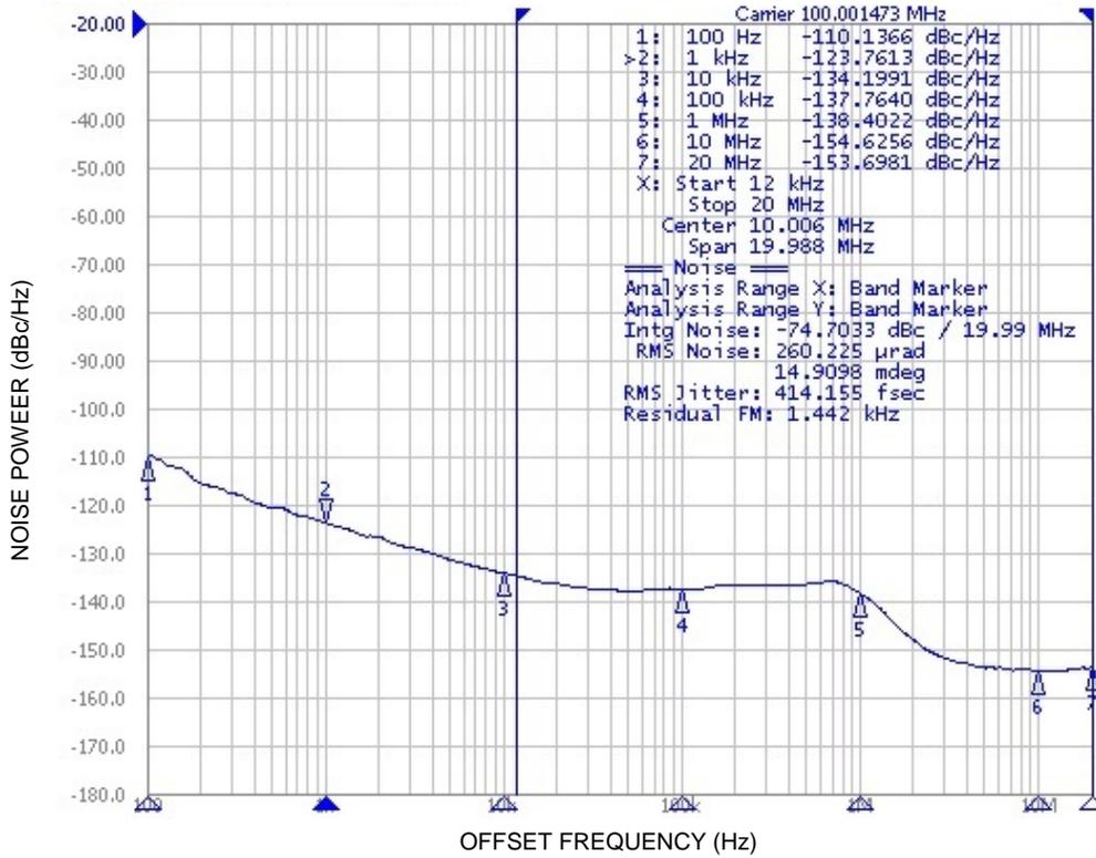
Figure 3. Typical Phase Noise Plot at 100 MHz; ( $f_{CLKIN} = 25$  MHz Crystal ,  $f_{CLKOUT} = 100$  MHz SS OFF, RMS Phase Jitter for Integration Range 12 kHz to 20 MHz = 414 fs, Output Termination = HCSL type)
