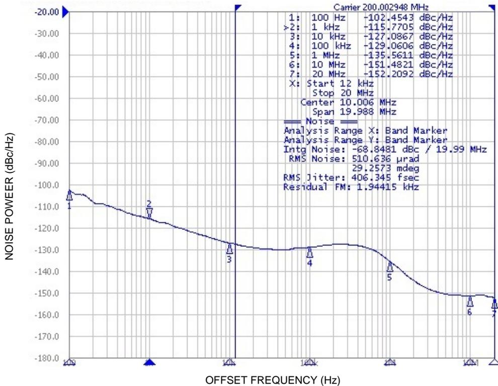
Figure 4. Typical Phase Noise Plot at 200 MHz; ( $f_{CLKIN} = 25$  MHz Crystal ,  $f_{CLKOUT} = 200$  MHz SS OFF, RMS Phase Jitter for Integration Range 12 kHz to 20 MHz = 406 fs, Output Termination = HCSL type)
